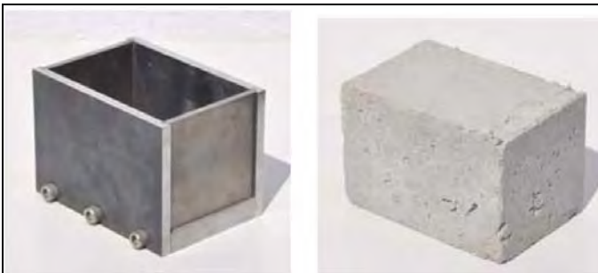
Figure 10. Partial beam box mold and test specimen.
