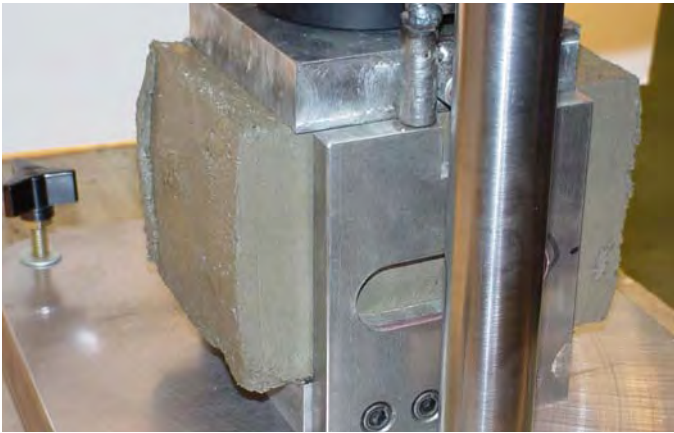
Figure 9. Shotcrete partial beam test specimen undergoing loading.
