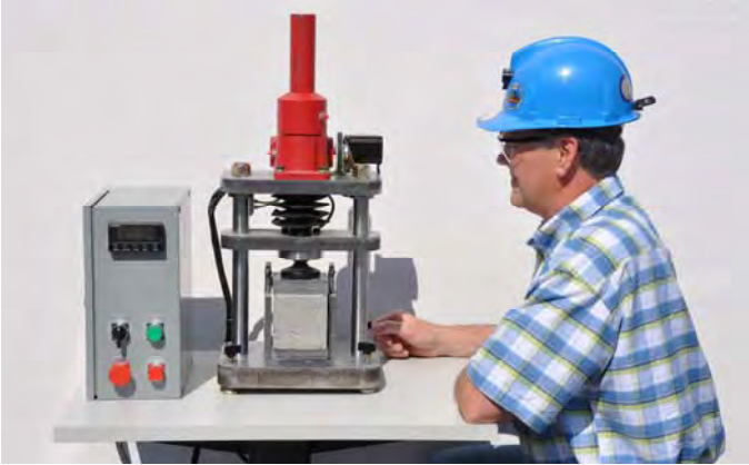
Figure 8. Early strength shotcrete test machine in operation.
