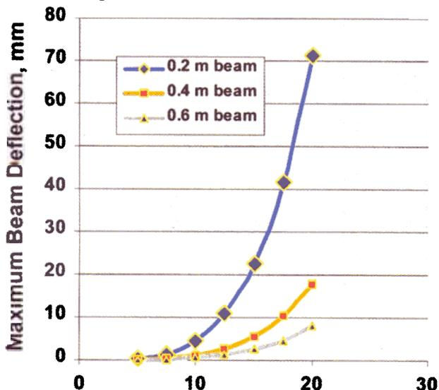
beams or plates. Figure 11 shows the effect varying beam lengths and thickness have on the maximum deflection of a 23.5 kN/m<sup>3</sup> (150 lb/cu ft), 41.4 GPa (6 million psi) fully intact beam of limestone. This deflection is small and can take place quickly after an opening is excavated. Or it can take place much later as weathering processes aid in forming new, thinner beams.
