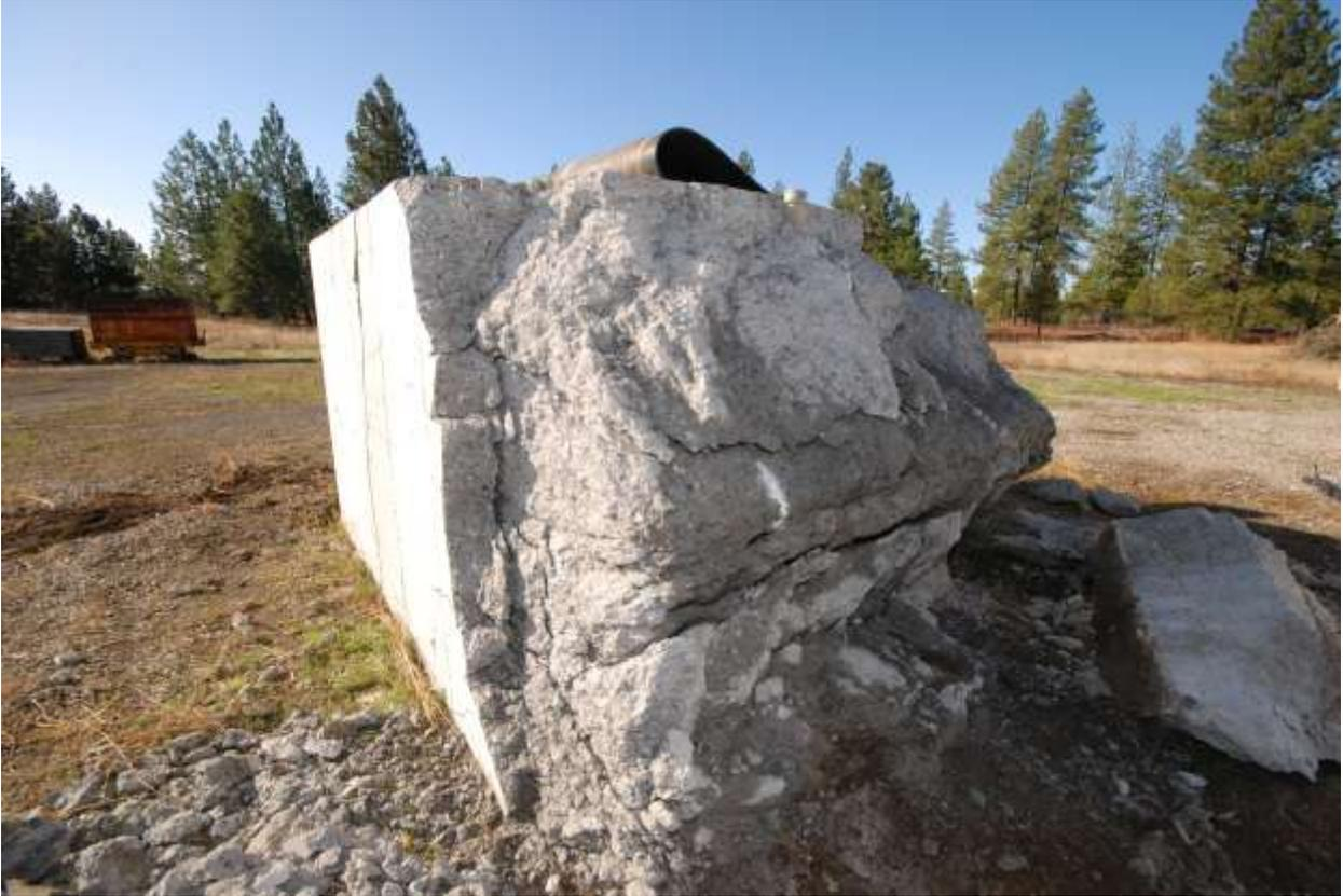
**Figure 13. Block 2 after blasting and prior to wire sawing showing remnants of blasthole location.**
