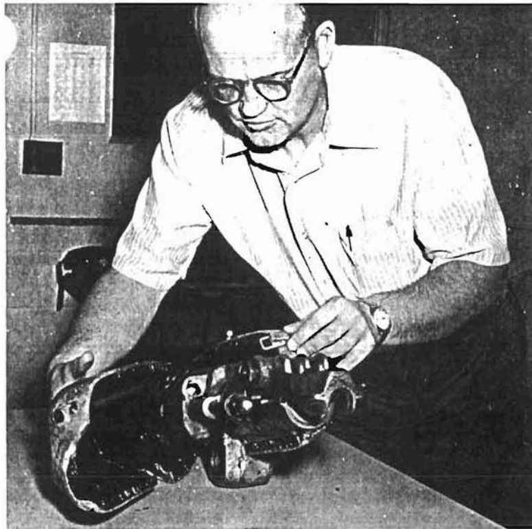
FIGURE 5. - Installation of plastic-aluminum-outer-surface muffler cover on Atlas-Copco BBC-17 drill.
