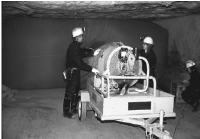
Figure 9.—The inflatable feed-tube partition deployed in the Lake Lynn Experimental Mine.
