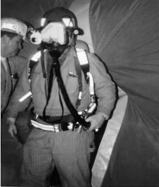
Figure 8.—Rescue team member wearing the Cairns IRIS and exiting the positive-pressure, inflatable escape device.
