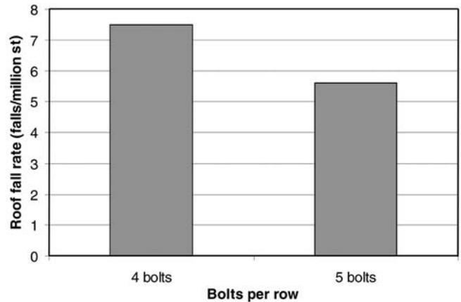
**Figure 11** — The effect of roof bolt pattern on the roof fall rate for Illinois Basin mines (2005 through 2006).
