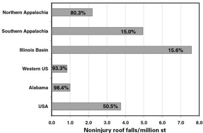
**Figure 2** — Roof-fall rates in selected coal basins in the United States (2005 through 2006).
