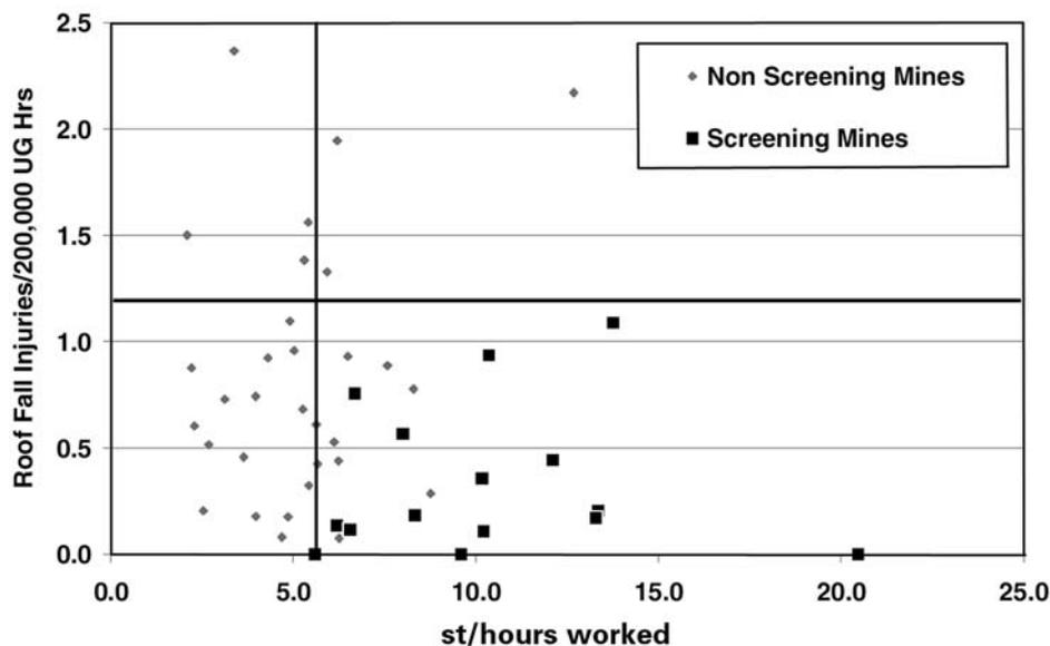
**Figure 15**— Safety and productivity in U.S. longwall mines that use roof screen vs. longwall mines that do not use roof screen (2003 through 2005).
