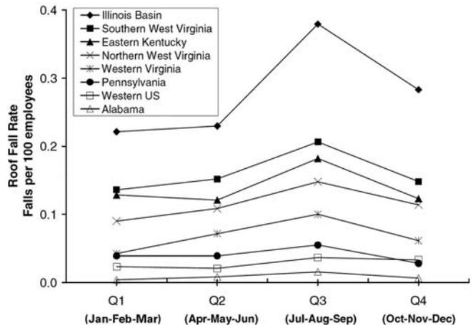
**Figure 4** — Seasonal roof fall rates for U.S. coal basins (2004 through 2006). The highest roof fall rates occur in the Illinois Basin during the summer months.
