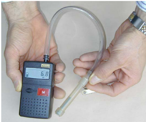
Figure 2. Respirable dust dosimeter showing pump with pressure readout and new plastic dust detector tube
