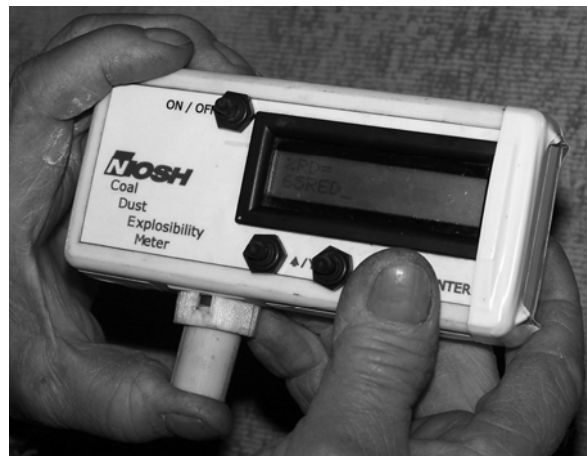
Figure 4: The hand-held coal dust explosibility meter (CDEM)
