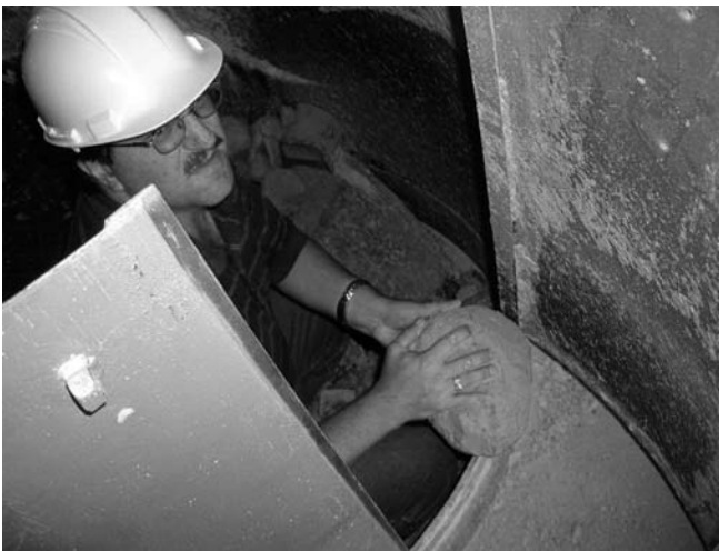
Figure 4b — Worker easily removing large rocks when using door.
