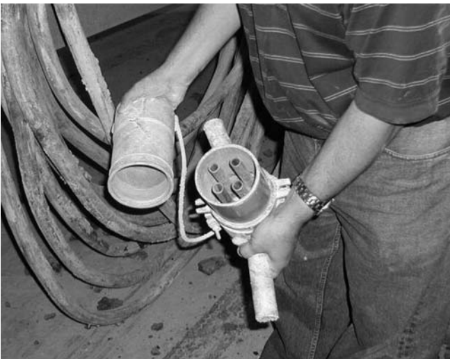
Figure 2 — The rubber “boot” to protect the male cable connector from dirt, dust and damage.
