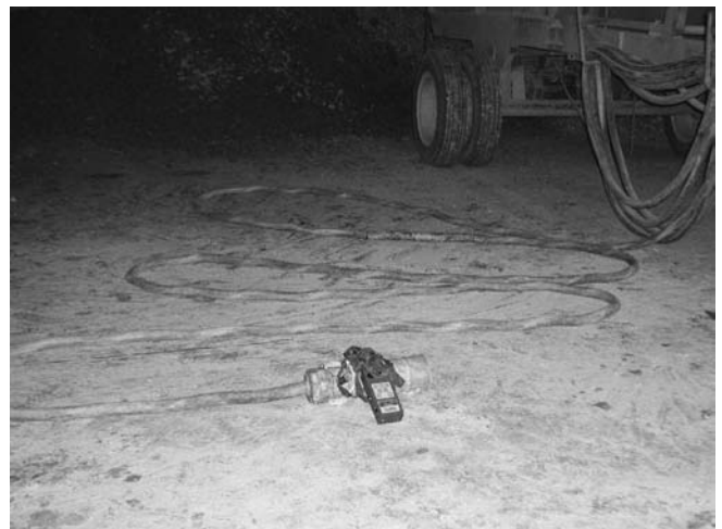
Figure 3b — Shredder cable evenly looped.
