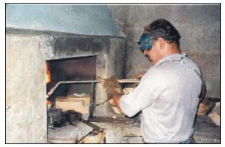
Following the processing of gold ore, a refinery worker in Bella Rica, Equador, burns the remaining impurities, which may lude small amounts of mercury.
