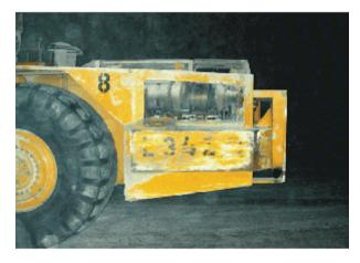
Diesel exhaust filtration on mining equipment offers substantial reductions in workplace DPM concentrations.
