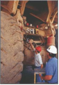
Mounting a collision warning device on the rear end of a haulage truck.
