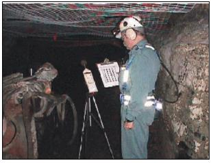
Noise profiling of underground mining equipment.
