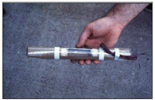
Explosive charge set up for the air gap test. This test evaluates the ability of the detonation of a permissible explosive to jump a gap in the explosive column.
