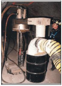
Inlet hood prototype for improved dust capture on drilling operations.
