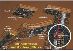
Stress monitoring system field tested for assessing coal bumps.
