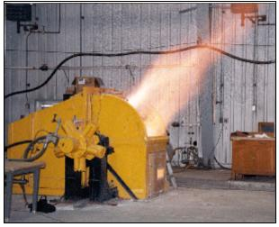
Frictional test apparatus showing ignition of methane-air.
