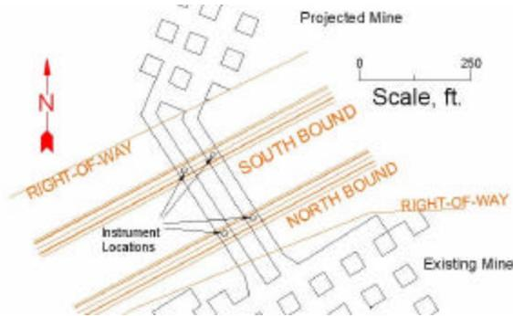
Figure 10. Map showing existing mine workings with projections.
