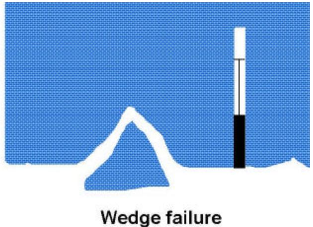
Figure 4. Monitor installation in wedge failure vicinity.
