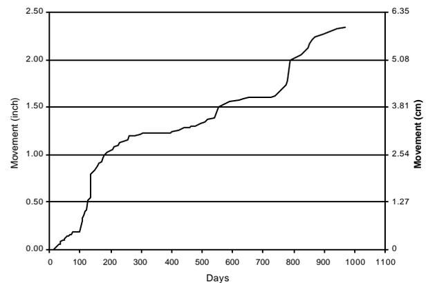
Figure 21. Roof movement at RMSS #27.
