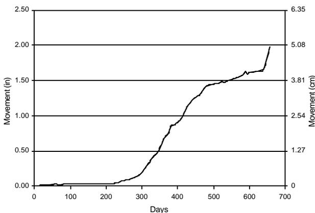
Figure 20. Roof movement at RMSS # 21.
