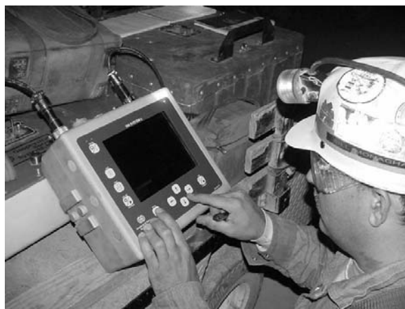
Figure 2. Photo of Engineer using the SIR-2 unit.
