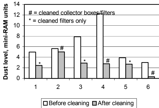
Figure 1. Dust levels before and after cleaning dust boxes and/or filters.
