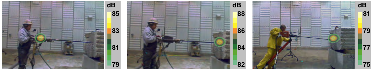
(j) S83 at 3150 Hz. (k) S83 w/muffler at 3150 Hz. (l) TE MD20 at 3150 Hz.
