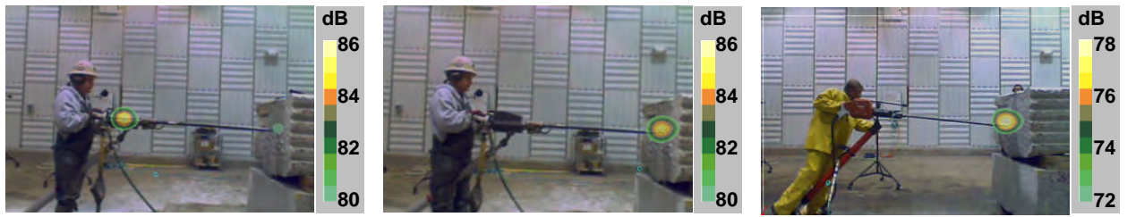
(m) S83 at 4000 Hz. (n) S83 w/muffler at 4000 Hz. (o) TE MD20 at 4000 Hz.
