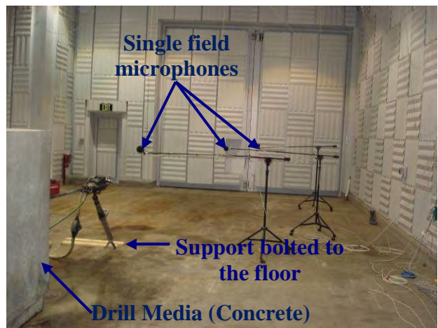
Fig. 2 - Experimental setup in the hemi-anechoic chamber for noise source identification, dose accumulation and single field microphone measurements.
