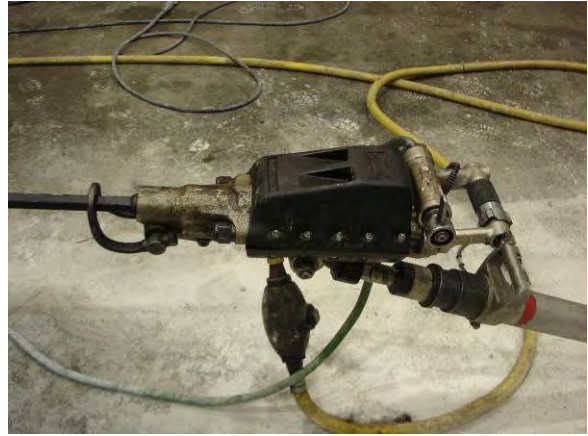
(b) Gardner Denver S83 with muffler.
