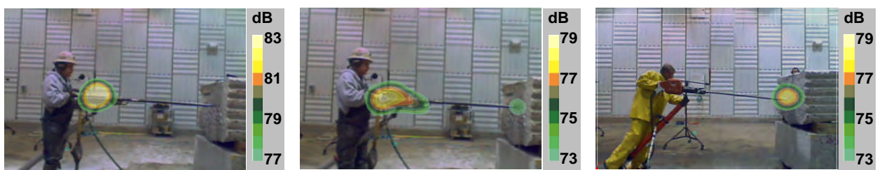
(g) S83 at 2500 Hz. (h) S83 w/muffler at 2500 Hz. (i) TE MD20 at 2500 Hz.
