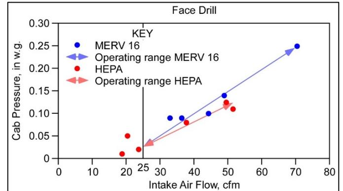
Figure 5. Comparing of intake airflow and positive cab pressure on the face drill with both the MERV 16 and HEPA quality filters.
