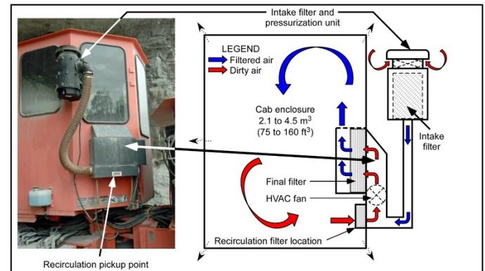
**Figure 2.** Actual filtration and pressurization unit on enclosed cab (left) and plan view design drawing and airflow pattern of the same unit (right).
