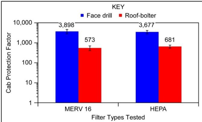
Figure 4. Average PF values for the face drill and roof-bolter machines comparing the MERV 16 and HEPA quality filters.
