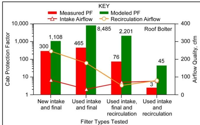
**Figure 6.** Roof-bolter cab performance changes with respect to different filters used in the system.
