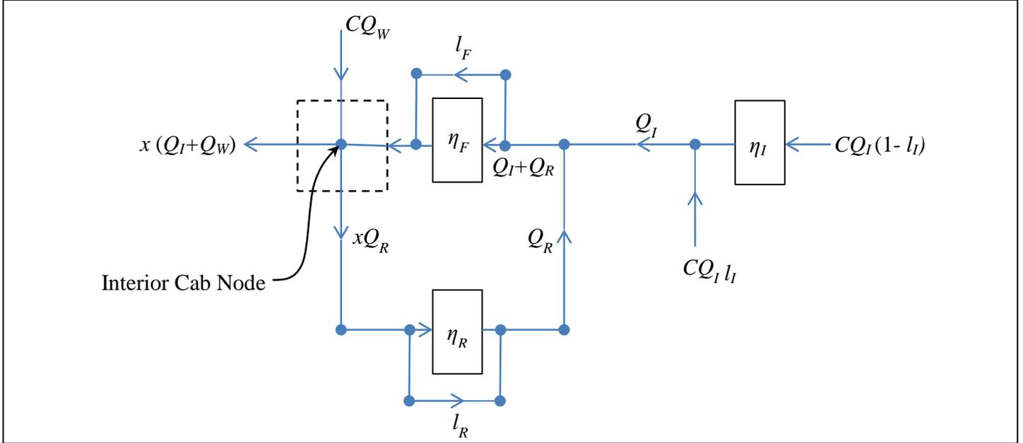
Figure A1. Three-filter cab system with potential leaks around the filters ( $Q$ 's denote air quantities,  $x$ 's &  $C$ 's denote contaminant concentrations, and  $\eta$ 's denote filter efficiencies).
