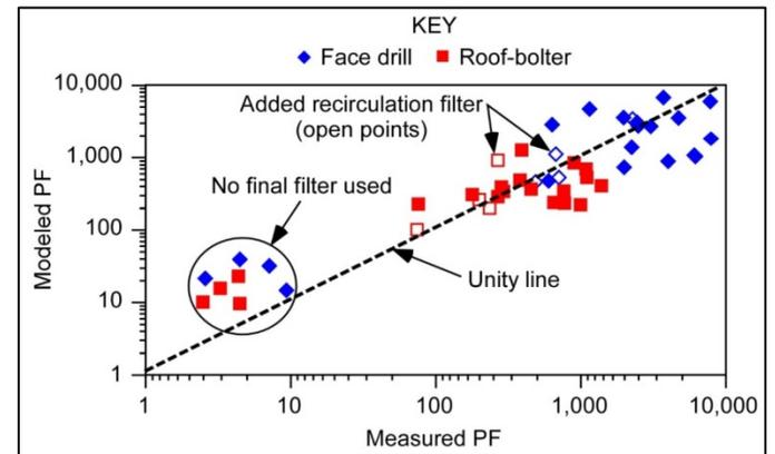
**Figure 7.** Measured and modeled protection factors of the face drill and roof-bolter during the filter field study.
