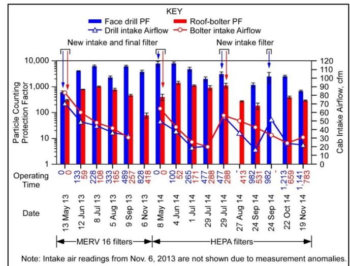
**Figure 3.** PF from particle count instruments for the enclosed cabs of the face drill and roof-bolter machines, as well as the intake airflow with MERV 16 as compared to HEPA filters.
