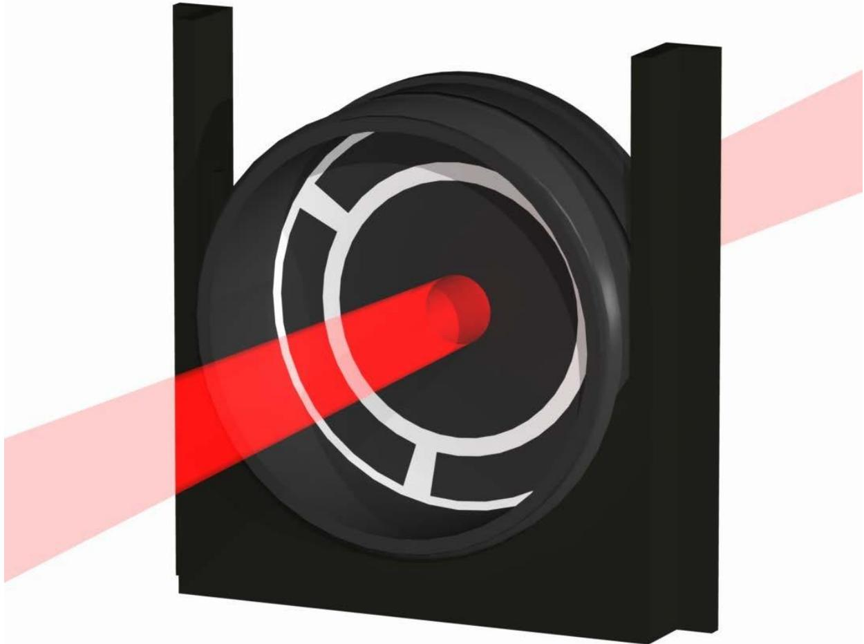
**Figure 5. Illustration of the relative position of the IR beam and sample cassette. When the sample cassette is correctly positioned in the instrument (within the removable cradle or filter holder), the IR beam will pass directly through the center of the sample at the focal point.**
