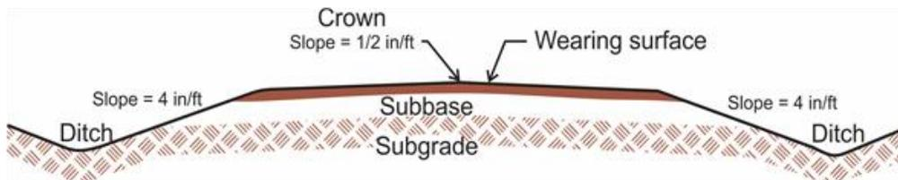
Figure 11.3. Illustration showing a cross section of a haul road.<sup>30</sup>
