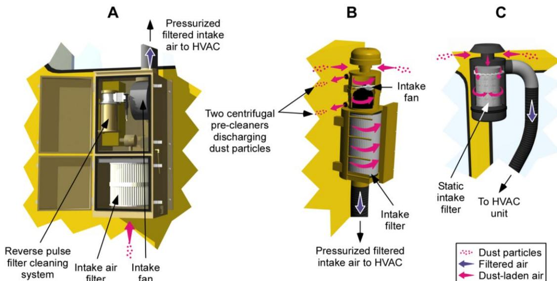
**Figure 10.8. Illustration of two types of recommended powered intake systems. A and B show a powered unit design (recommended) while C shows a static, non-powered system (not recommended).**
