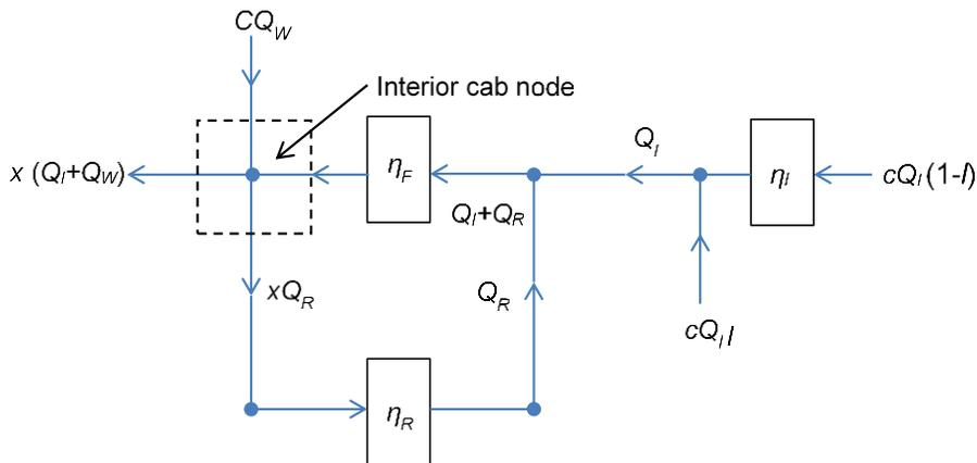
**Figure 10.4. Three-filter cab system with the final filter downstream of the intake and recirculation filters. Q’s denote air quantities, x’s & c’s denote contaminant concentrations, and η’s denote filter efficiencies.**
