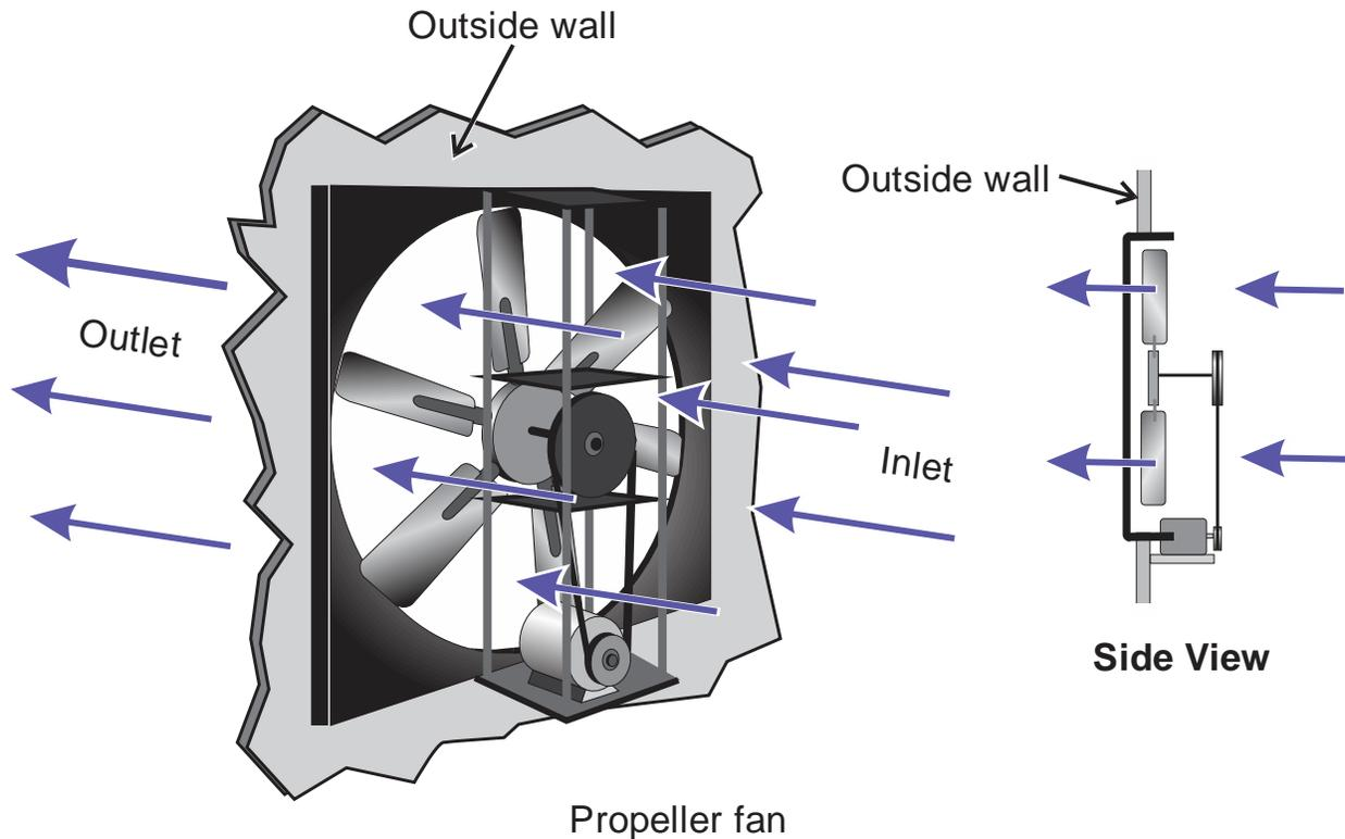
**Figure 2.29. Illustration of a wall-mounted propeller fan.**
