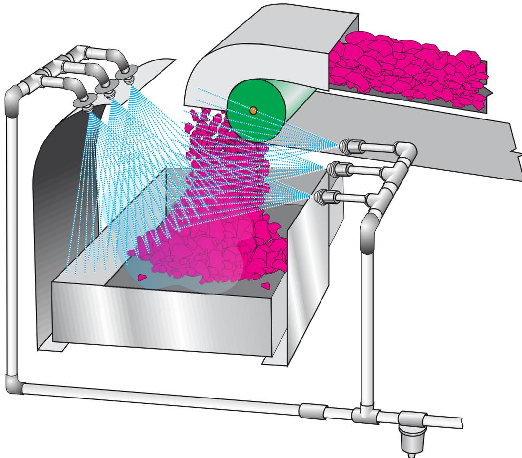
**Figure 3.2. Common dust control application illustrating nozzle positioning.**
