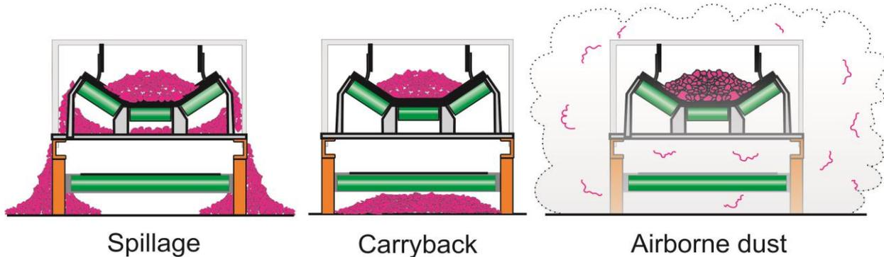
**Figure 6.2. Illustration of types of fugitive emissions from conveyor belts.**
