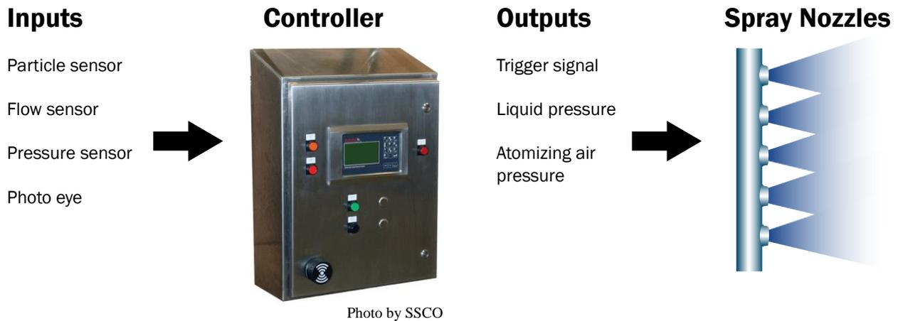
**Figure 3.19. Components of a typical automated control system. Arrows indicate flow of the system logic. Inputs feed into the controller and the controller feeds outputs to affect the operation of the nozzles [adapted from SSCO 2018].**
