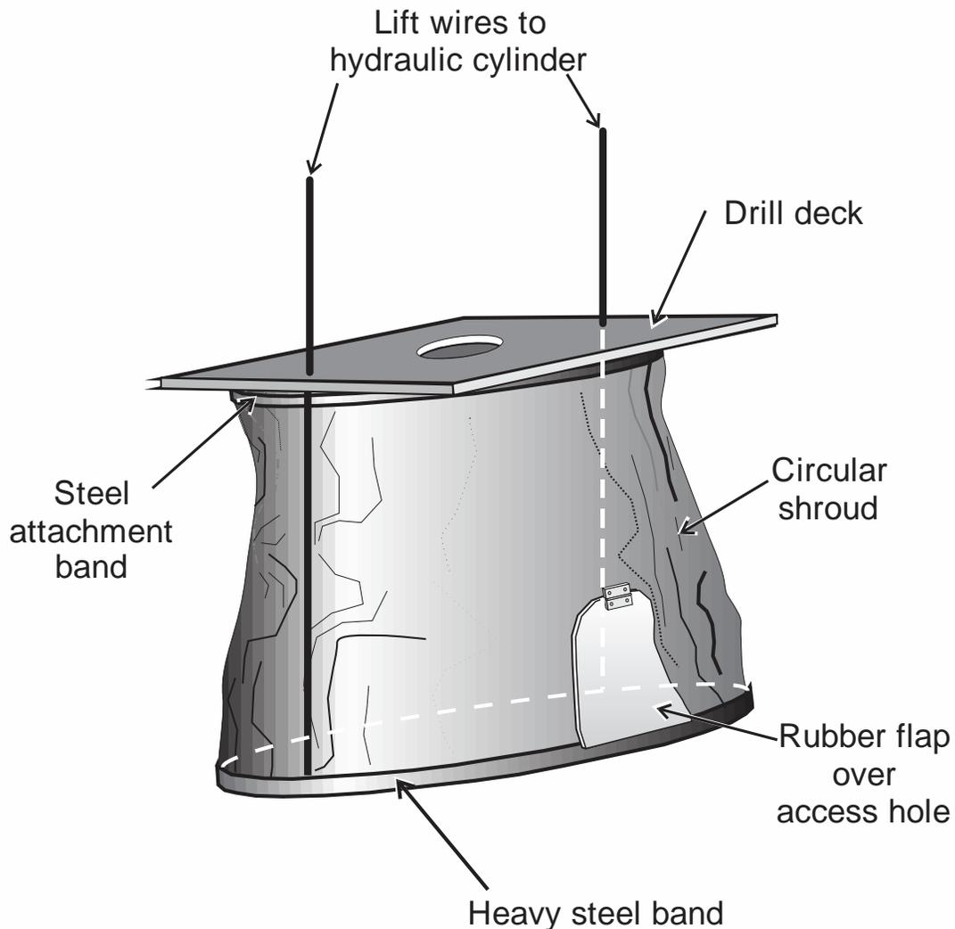
**Figure 4.6. Illustration of a circular shroud design.**
