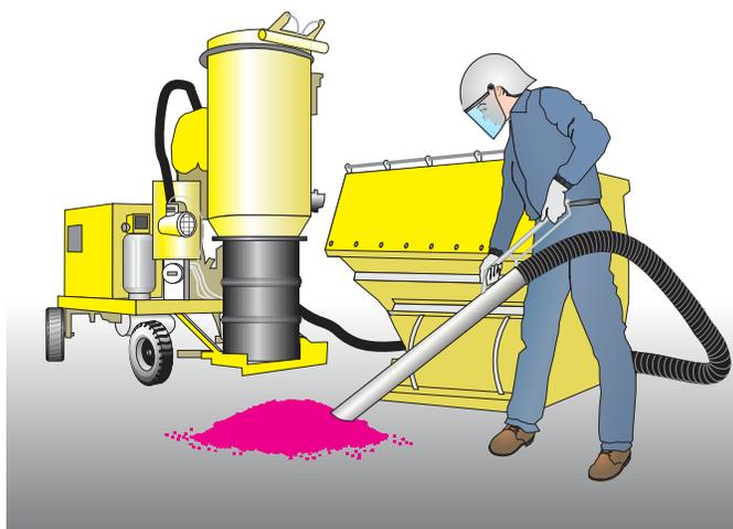
**Figure 9.19. Illustration of a portable system used to vacuum product.**
