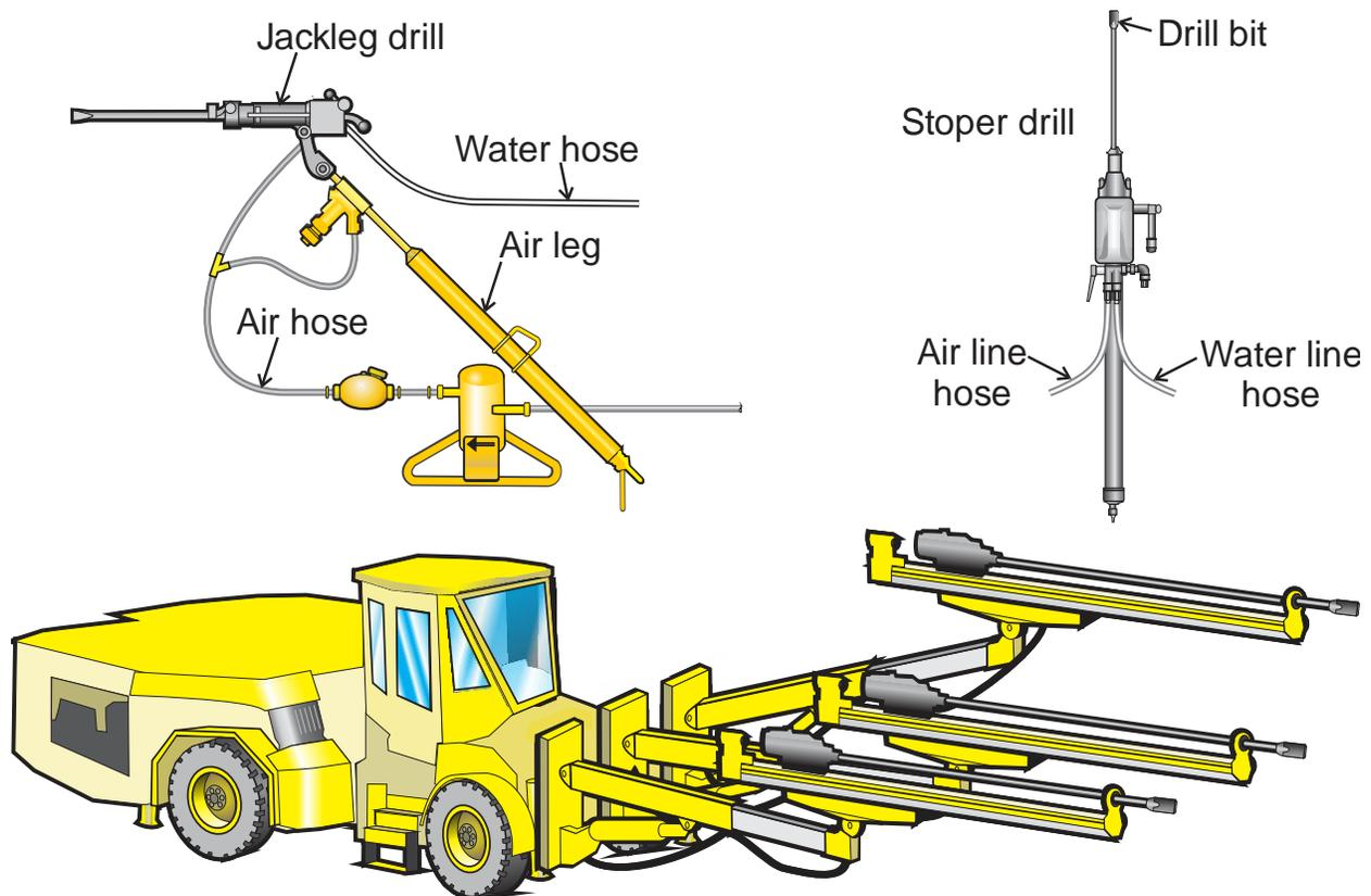
**Figure 4.19. Illustrations of three types of drilling equipment. A typical jackleg drill is shown on the top left, a stoper drill on the top right, and a three-boom jumbo on the bottom.**
