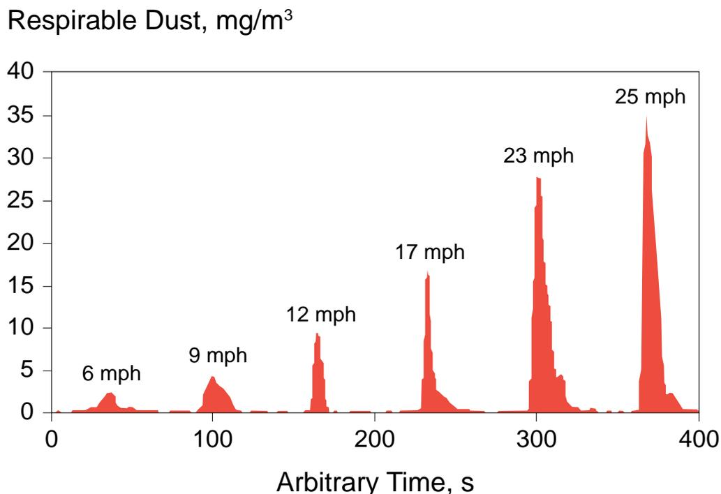
Figure 11.2. Graph showing a dust profile measured at roadside for a haul truck traveling at various speeds (mph) [adapted from Thompson and Visser 2001].
