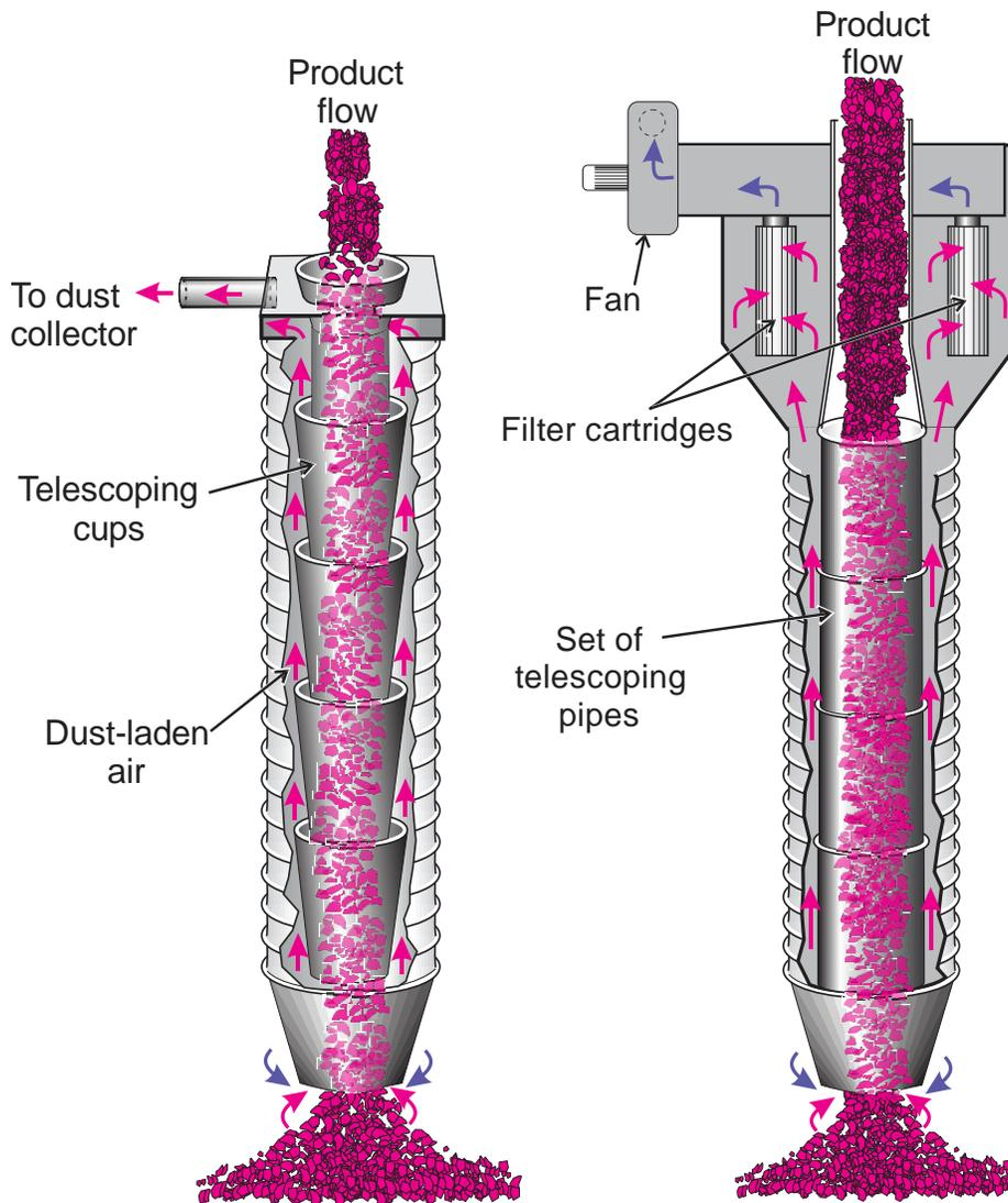
**Figure 8.1. Illustration of loading spouts designed with telescoping cups or pipes and dust collection capabilities.**
