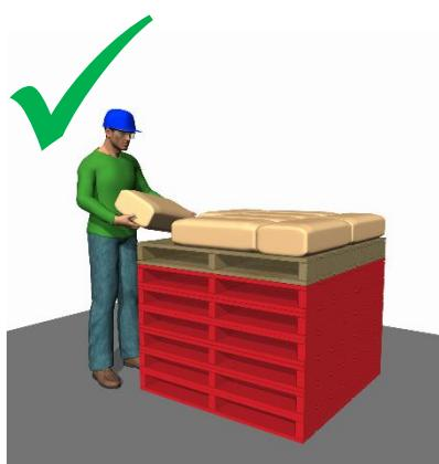
**Alternative Solution:** If a rotating lift table is too expensive, raise the height of the lower pallet by creating a stack of supporting pallets. Then, palletize the bags mid-height before removing the pallet from the stack and continue to palletize the already stacked pallet on the floor.
