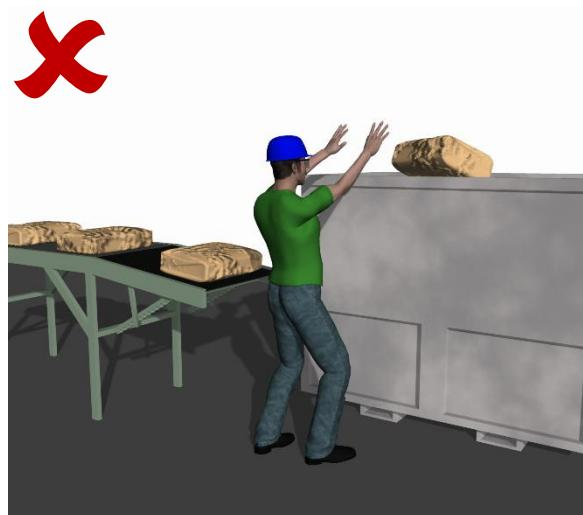
**Problem:** When scrap materials need to be moved from conveyors to dumpsters with a high lip, the material may need to be lifted at or above shoulder height and lead to musculoskeletal injuries.
