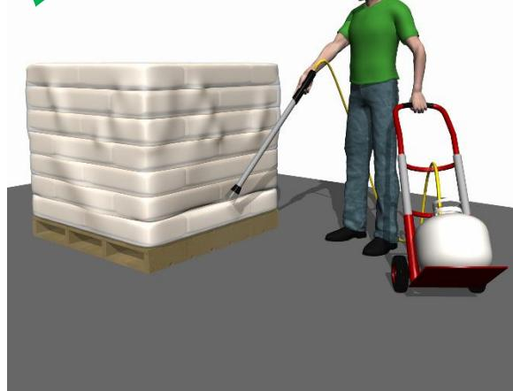
**Solution:** Supply a wheeled cart for the propane tank. This allows the worker to pull the cart instead of manually carrying the tank, which may weigh over 20 lbs.
