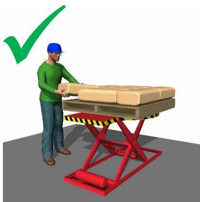
**Solution:** Provide a self-adjusting lift table to improve access and safety by ensuring workers are working near elbow height. When possible, use a rotating lift table to reduce reaching to access the differing areas on the pallet.
