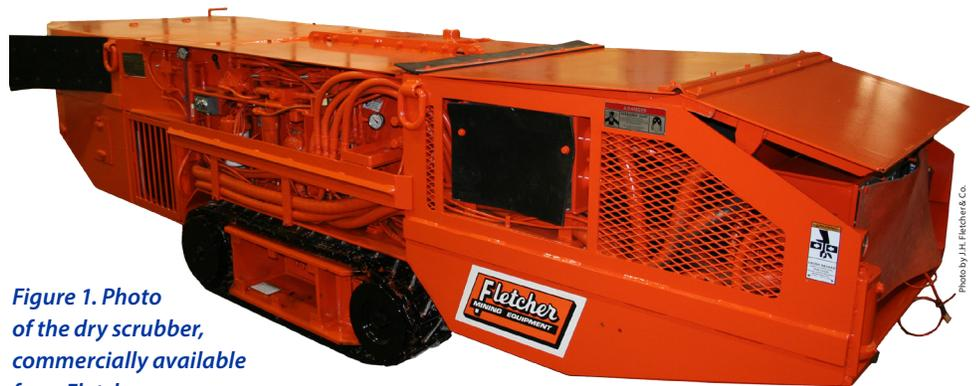
*Figure 1. Photo of the dry scrubber, commercially available from Fletcher.*
