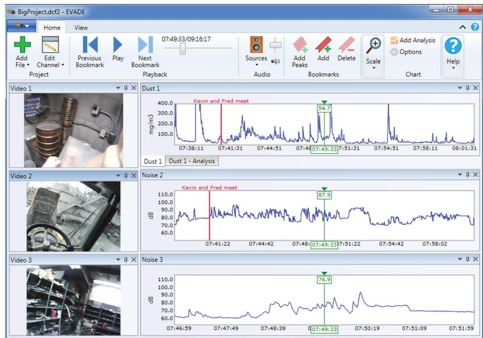
This screenshot from the EVAD 2.0 software shows the expanded multi-channel capabilities of the program. In this example, three separate video channels have been created and are displayed next to their associated exposure plots.
