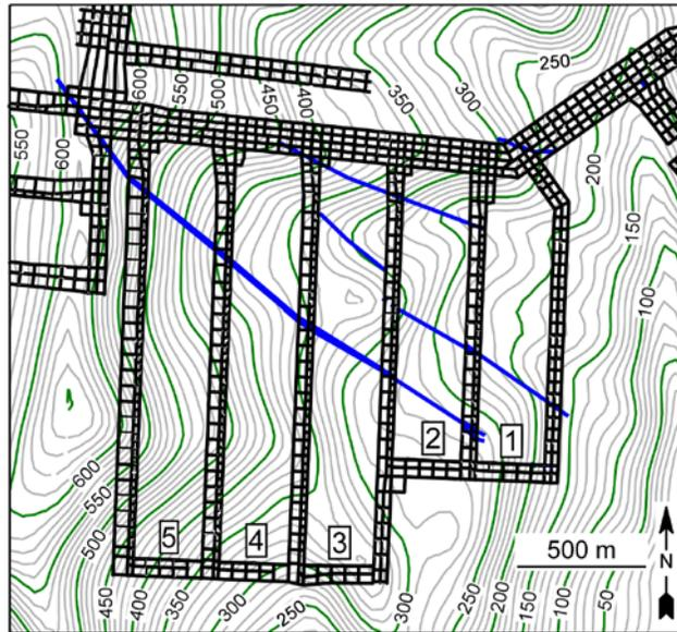
**Figure 28. Map showing a five-panel longwall section traversed by several steeply dipping faults (blue lines).**
