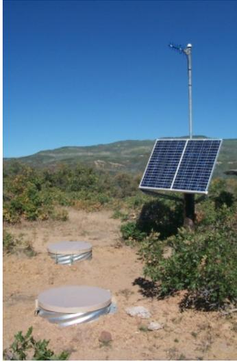
**Figure 25. Seismometer, remote power, and telemetry infrastructure of a typical district-wide network station.**
