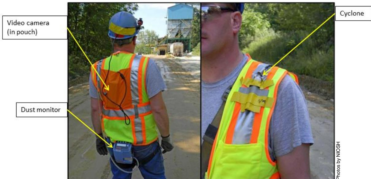
**Figure 3. Setup of sampling devices for personal sampling.**
