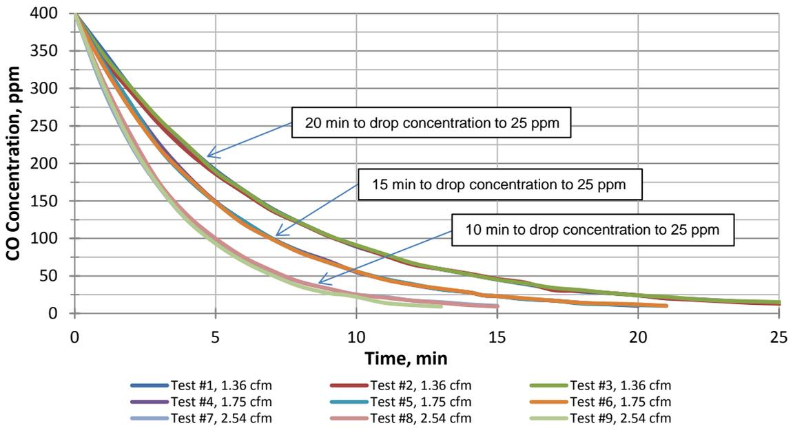
**Figure 2. Mini purge box test results at 0.53 psig relief pressure and three different purge air flow rates.**
