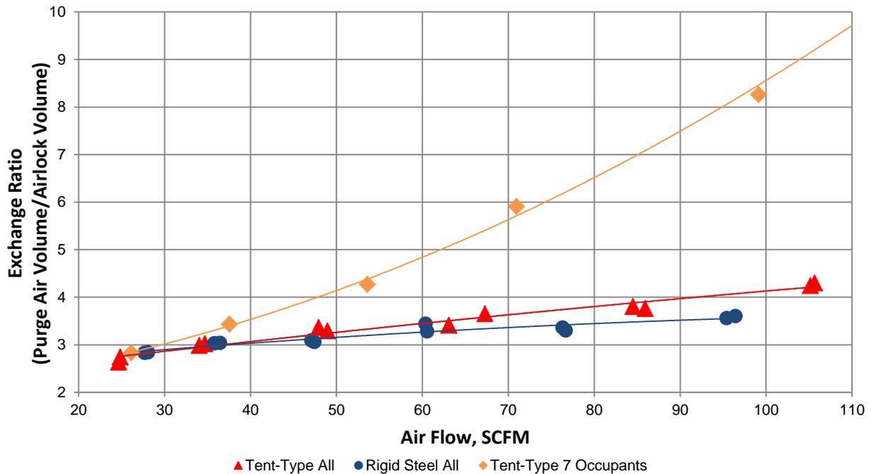
**Figure 13. Graph of exchange ratio versus air flow for the tent-type and rigid steel mobile refuge alternative airlocks.**
