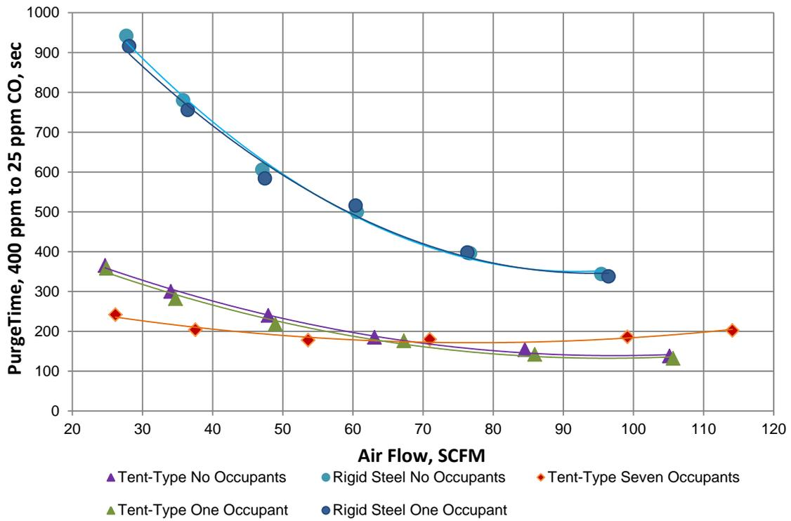
Figure 11. Graph of time required to purge versus air flow rate.
