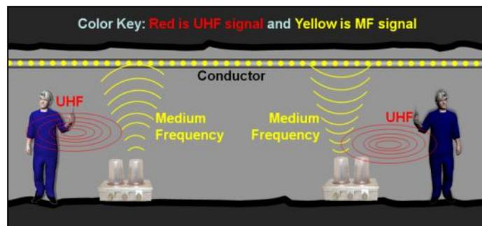
**Figure 3.** A simple example of an MF-to-UHF bridge.
