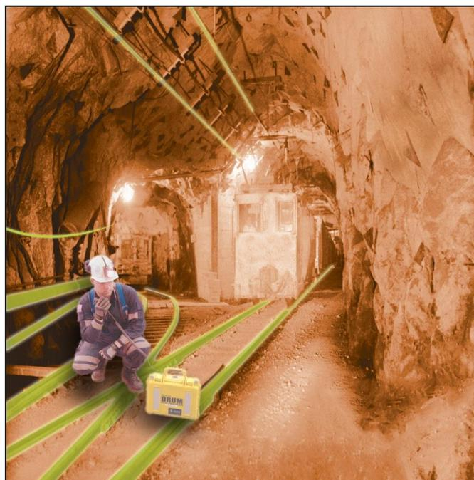
**Figure 1.** Medium frequency (MF) communications on existing conductors (highlighted green) in a mine.
