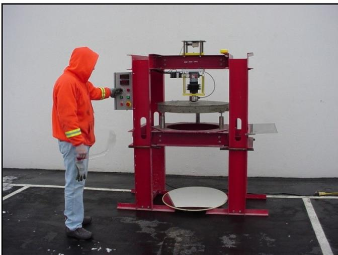
Figure 1. Portable round determinate panel test system.
