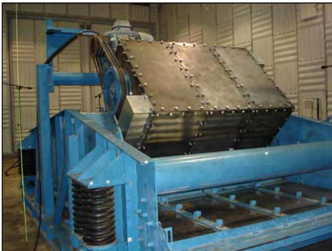
Figure 3.—Completed mechanism enclosure.
