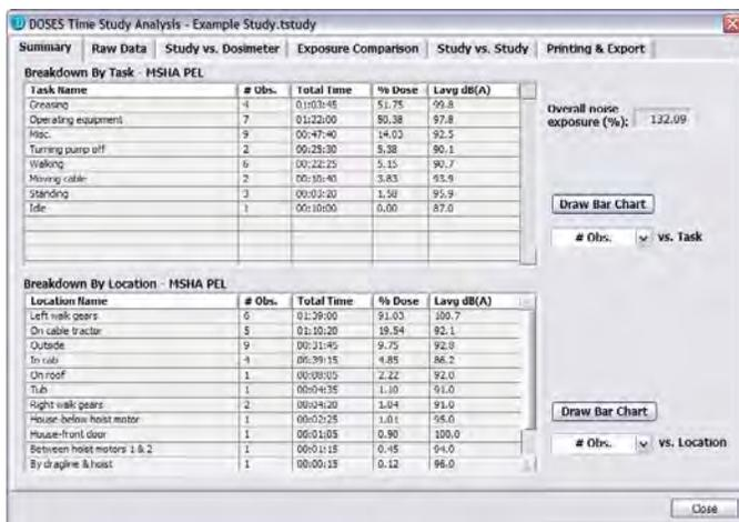
**Figure 2.—The first tab in the Analysis dialog showing the breakdown by task and location tables.**
