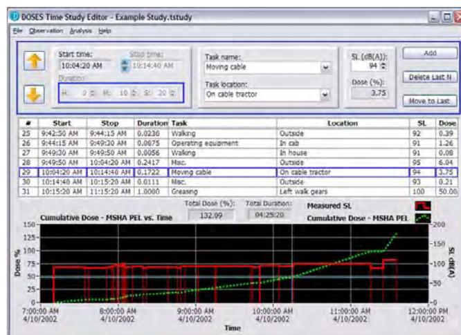
Figure 1.—The DOSES Time Study Editor with areas for entering new or editing existing observations, a table displaying the observations, and a graphical plot of cumulative dose and sound level versus time.
