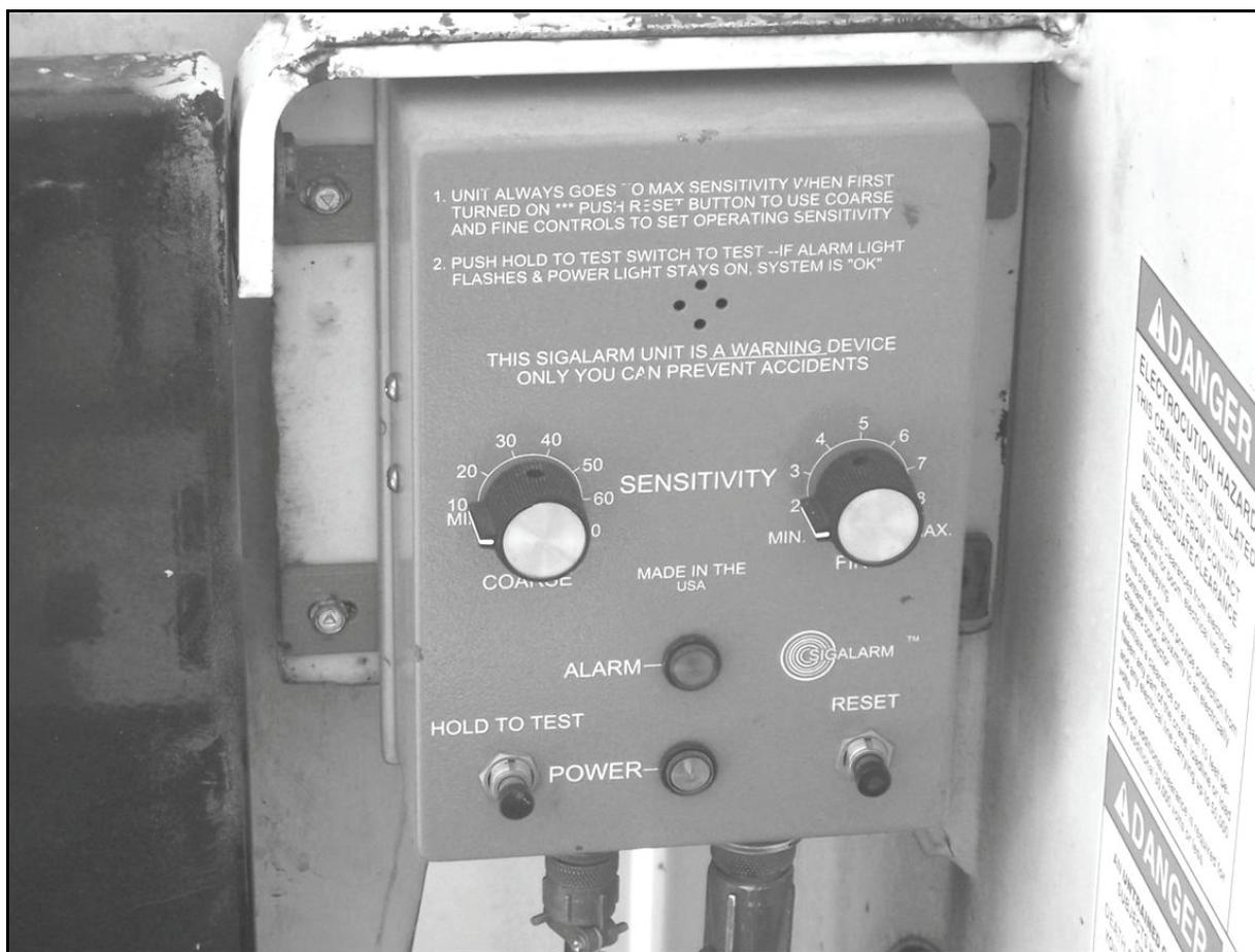
Figure 1.—SIGALARM Model 210 control unit.
