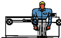
You can see here that the way equipment is designed does not always consider the worker using it. Workers are often put in situations where their tools and equipment are designed so that they must get into awkward positions (reaching and stooping) in order to operate the equipment.
