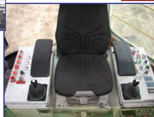
Dragline operators were complaining of upper-extremity discomfort and pain. It was determined that the support and function of the manufacturer-installed armrests were inadequate and nonadjustable. The new armrests were adjustable and provided larger nonfrictional support.
