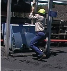
**TASK DESCRIPTION:** The electromagnet is manually pulled to the scrap bin by pulling down on a chain over a pulley. The magnet is heavy, and maximum effort is required. The worker reaches to his maximum height to grasp the chain and pull down using his entire body weight.
