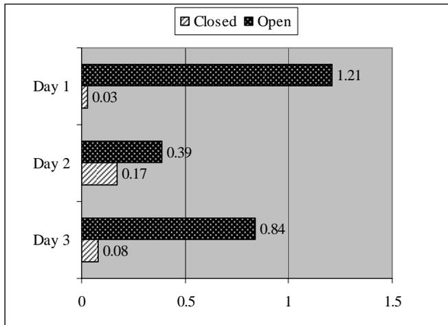
**Figure 2.—Average respirable dust concentration (mg/m<sup>3</sup>) inside drill cab during periods with the cab door closed and open for 3 days of testing.**
