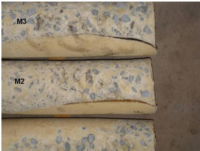
Figure 18.—Separation along the interface between lifts observed in 6-in-diam core drilled horizontally. The right side of the cores is the front side of the seal.
