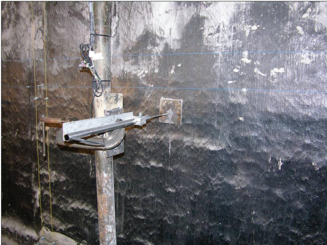
Figure 4.—LVDT mounted behind seal to measure movement of the seal during an explosion. The vertical yellow wires to the left of the sensor post and the horizontal blue wires above the LVDT anchoring plate on the seal are the breakwires.
