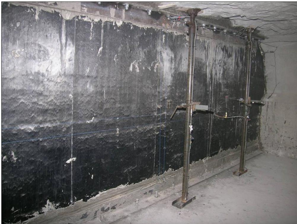
**Figure 23.—Completed CFRP reinforcement retrofit to the C-320 pumpable cementitious foam seal, and the LVDT displacement sensors mounted to posts and attached to seal.**
