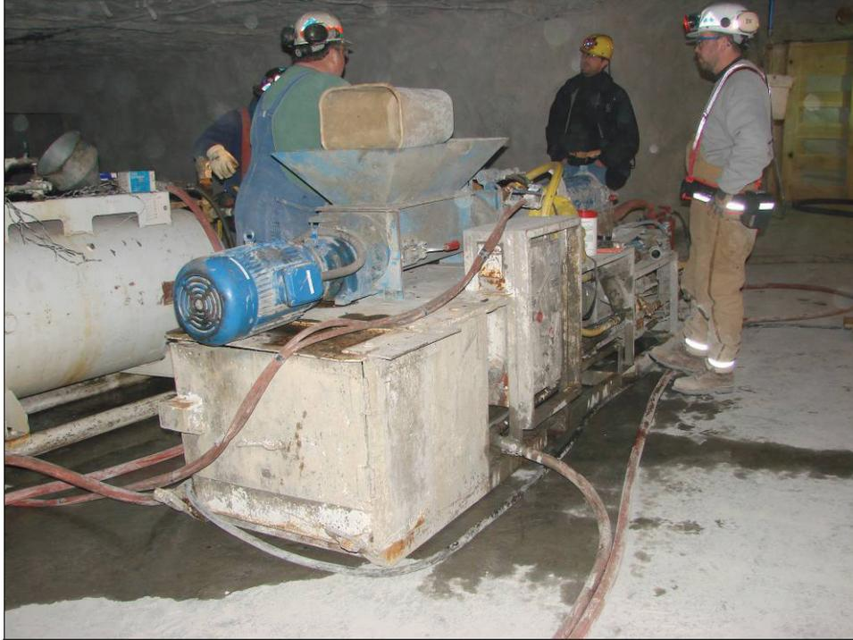
**Figure 8.—Electric-powered screw auger (*center of photo*) for the cement feed and the heated water and foam tank (*left side of photo*).**
