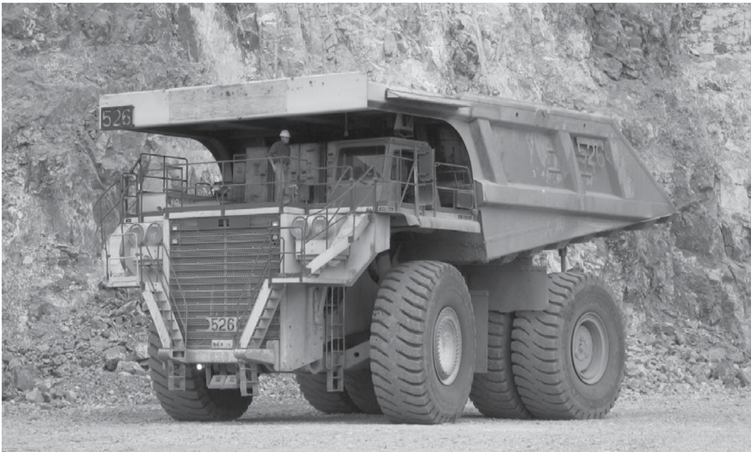
Figure A.1. Euclid EH4500 280-ton-capacity haul truck.
