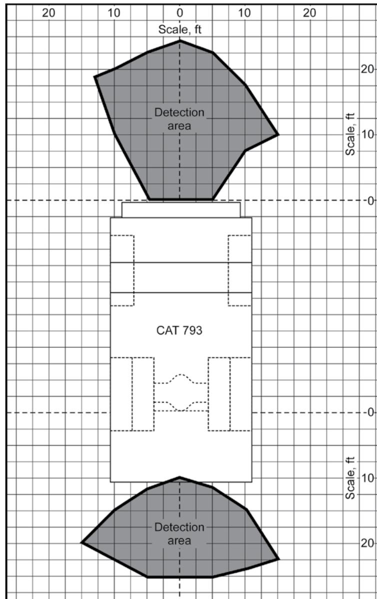
**Figure 8.** Preco radar detection areas for a person.
