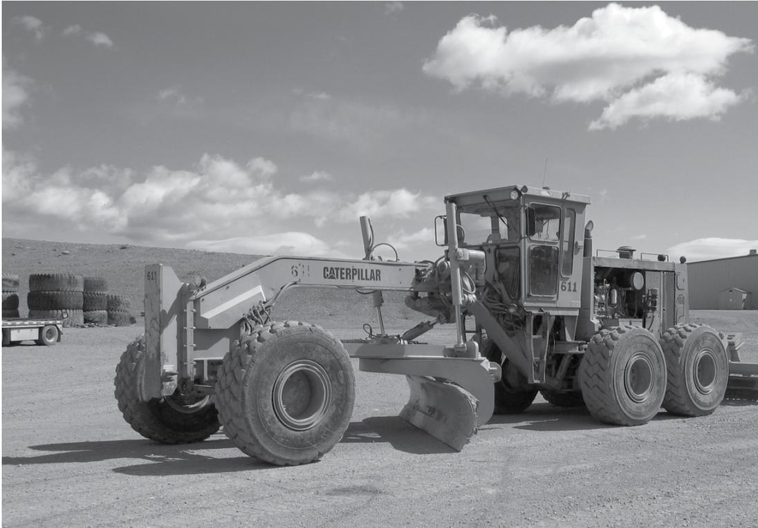
Figure A.13. Caterpillar 16G motor grader.
