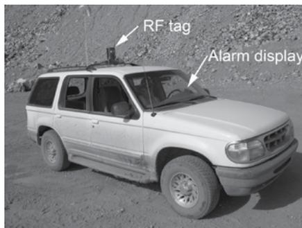
**Figure 15.** AMT RF tag mounted on a passenger vehicle.
