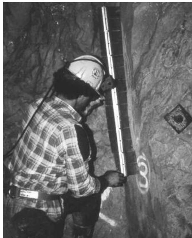
**Figure 3.—One-meter-long profile comb used to measure discontinuity roughness at 10 mines across Canada.**
