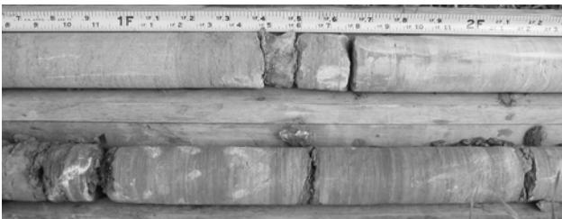
**Figure 1.—Photograph of core showing different rock layers and a prominent clay layer from 1.4 to 1.5 ft.**
