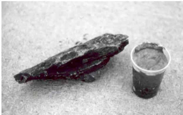
**Figure 1.—Effect of water on a moisture-sensitive shale.**
