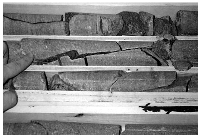
**Figure 10.—Joint geometry may not be obvious from the drill core unless the joint is intersected at a very shallow angle.**
