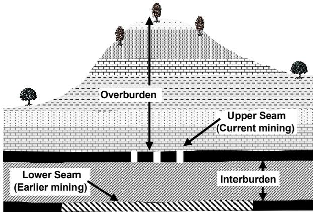
Figure 3.—Overmining interaction.
