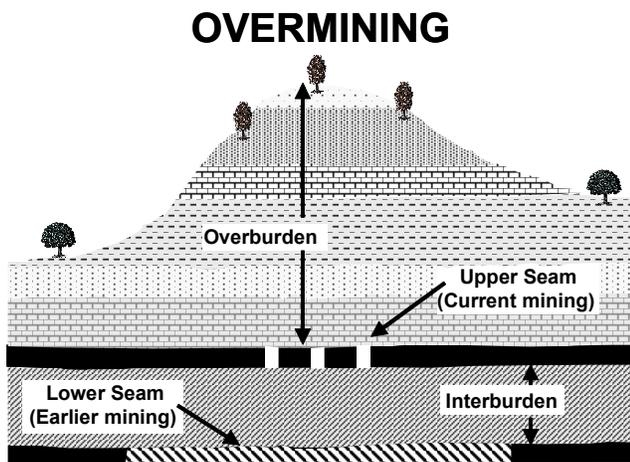
Figure 5.—Overmining interaction.
