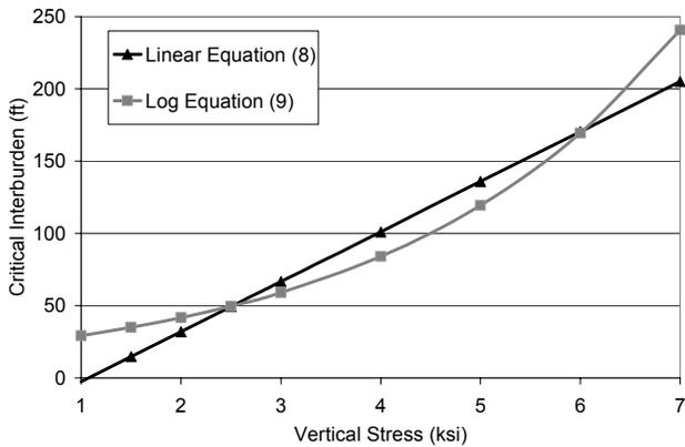
**Figure 13.—Comparison of Equations 8 and 9, showing that the logarithmic version (Equation 9) can yield the most conservative value of the critical interburden when the calculated interburden is less than about 50 ft.**
