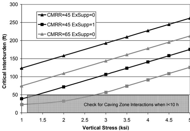
Figure 18.—Suggested values of the critical interburden for overmining a gob-solid boundary.
