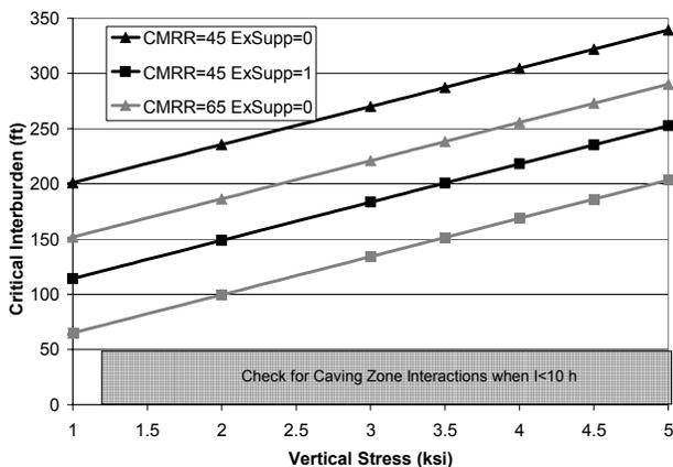
Figure 19.—Suggested values of the critical interburden for overmining an isolated remnant pillar.
