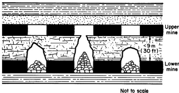
Figure 7.—Ultraclose mining (after Chekan and Listak [1994]).
