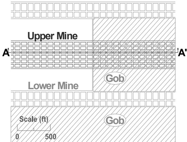
Figure 10.—Idealized mine plan for the case study analysis.
