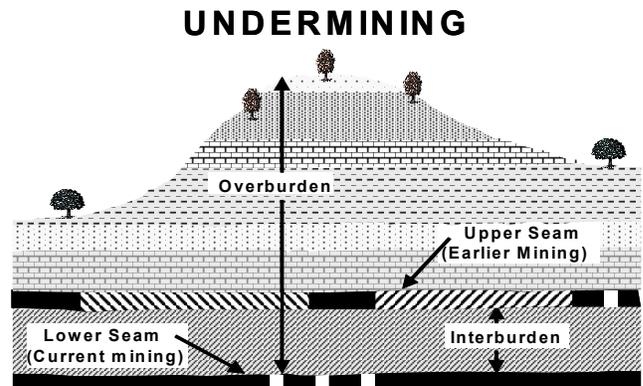
Figure 3.—Undermining interaction.
