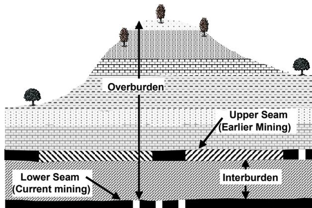
Figure 2.—Undermining interaction.
