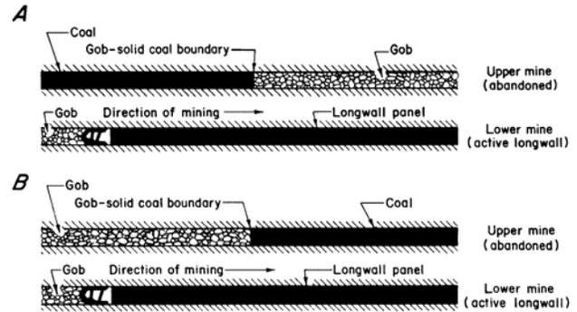
**Figure 9.—Influence of retreat direction on multiple-seam interaction: (A) retreating from solid to gob creates an unfavorable “stress window,” while (B) retreating from gob to solid results in lower stress concentrations (after Chekan and Listak [1993]).**
