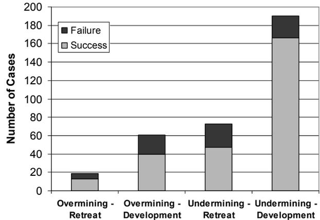
Figure 4.—Histogram showing the case history database by type of mining (development or retreat) and type of interaction (overmining or undermining).
