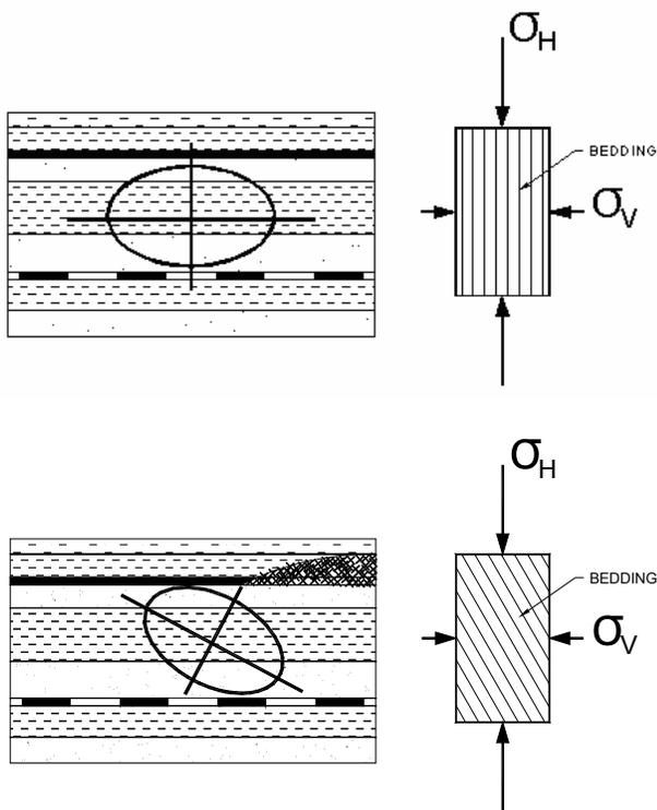
**Figure 14.—Reorientation of principal stresses leads to failure due to multiple-seam mining interaction. In single-seam mining, far-field principal stresses are generally aligned parallel to the bedding planes in which a test specimen is relatively strong. If the far-field principal stresses are rotated due to nearby multiple-seam mining, the bedding planes are oriented in an unfavorable direction in which a test specimen is relatively weak.**
