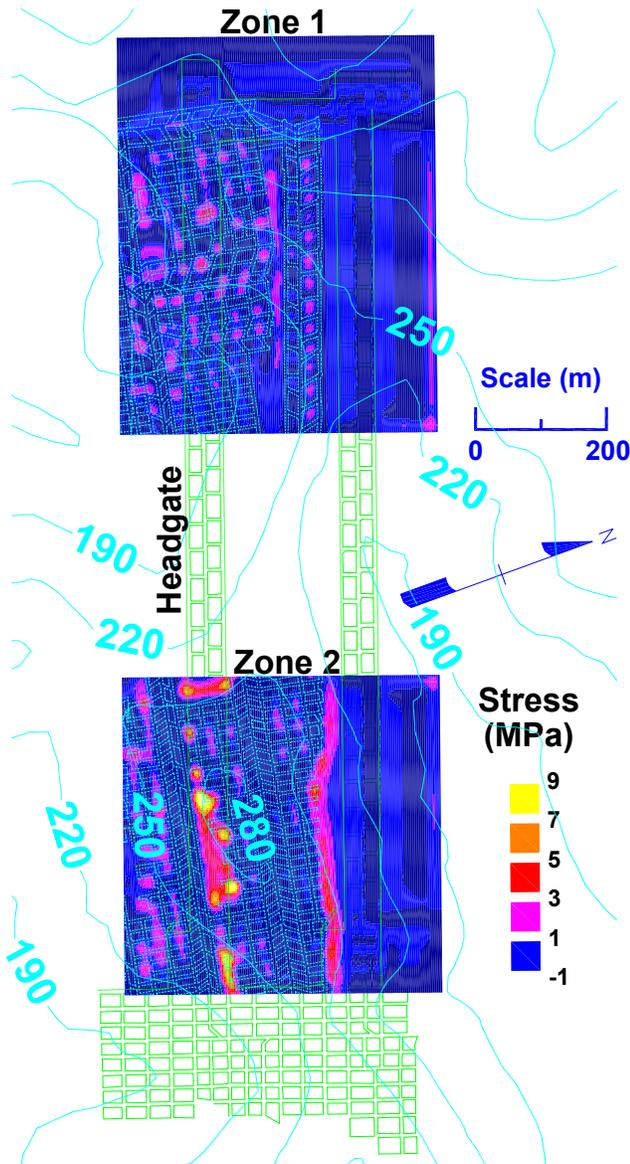
Figure 4.—Interseam stress for Zone 1 and Zone 2.
