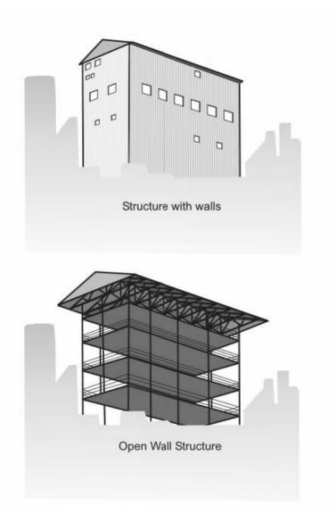
Figure 6.—Comparison of walled and open structure design for same size mineral processing building.
