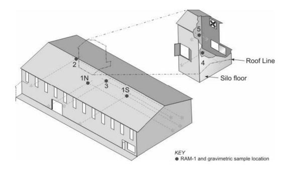
Figure 4.—Dust and noise sampling instrumentation setup at steel-sided structure No. 3.
