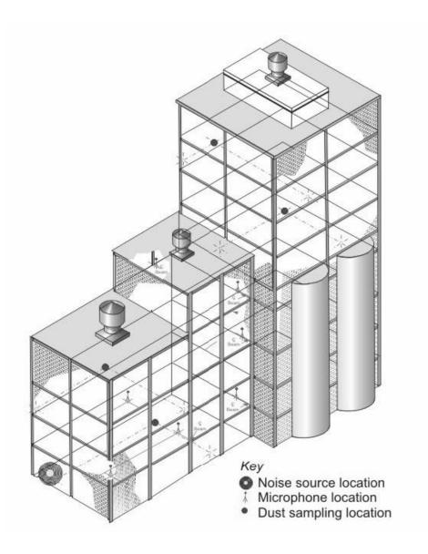
Figure 1.—Dust and noise sampling instrumentation setup at masonry structure No. 1.
