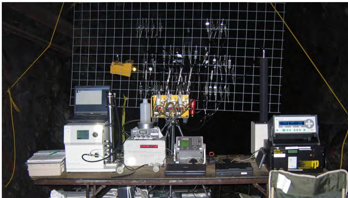
**Figure 8.—Downstream sampling station showing instrumentation and wire grid supporting DPM samplers, anemometer, iTX gas monitor, and RKI Eagle CO<sub>2</sub> monitor.**
