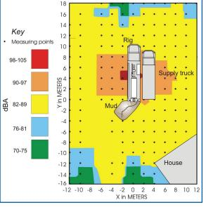
**Figure 1.** The image above shows sound levels around a typical water well worksite. In this example, workers are exposed to sound levels above 90dB(A) within 6 meters of the rig, particularly near the compressor. All workers at a worksite should always wear hearing protection and avoid standing in these areas if not required to conduct a work task.
