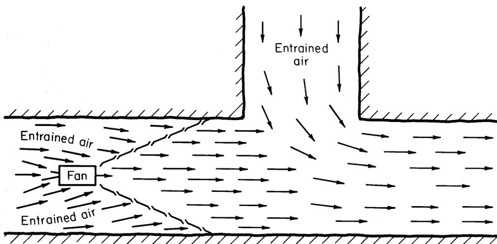
Figure 4-3.—Jet fan entrainment of mine air.
