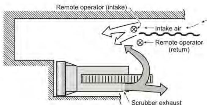
Figure 2-2.—Dust scrubber used with blowing ventilation.
