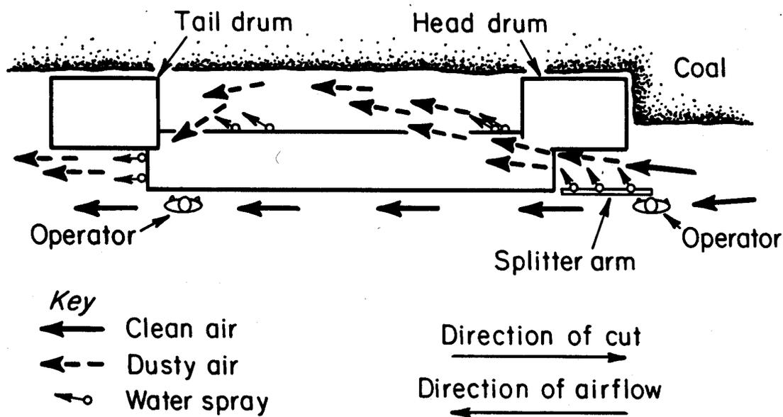
Figure 3-4.—Air currents when using the shearer-clearer system.
