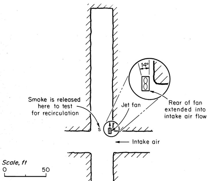
Figure 4-2.—Jet fan ventilating a single straight heading.
