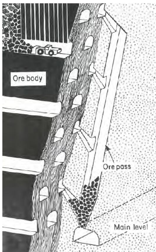
**Figure 6-1.—Ore pass adjacent to steeply dipping ore body. (Courtesy of the Society for Mining, Metallurgy, and Exploration (SME) ([www.smenet.org](http://www.smenet.org).)**
