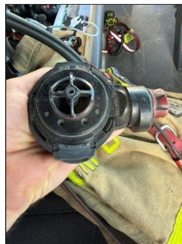
An SCBA regulator with integrated microphones. Photo by NIOSH
