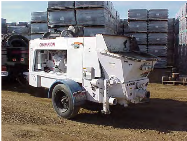
Figure 92. Swing-type, positive-displacement pump used to apply wet mix shotcrete.
