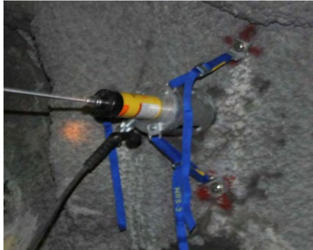
Figure 59. Pulling unit mounted to mine rib using a three-point safety restraint.
