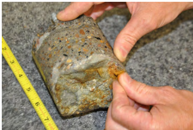
Figure 70. Test core #3: tensile failure in weak host rock.
