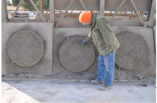
Figure 76. Sprayed round-panel shotcrete samples.
