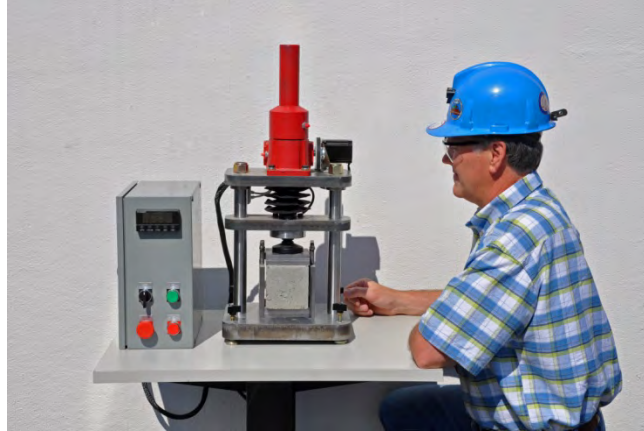
Figure 35. Operation of portable shotcrete test machine.
