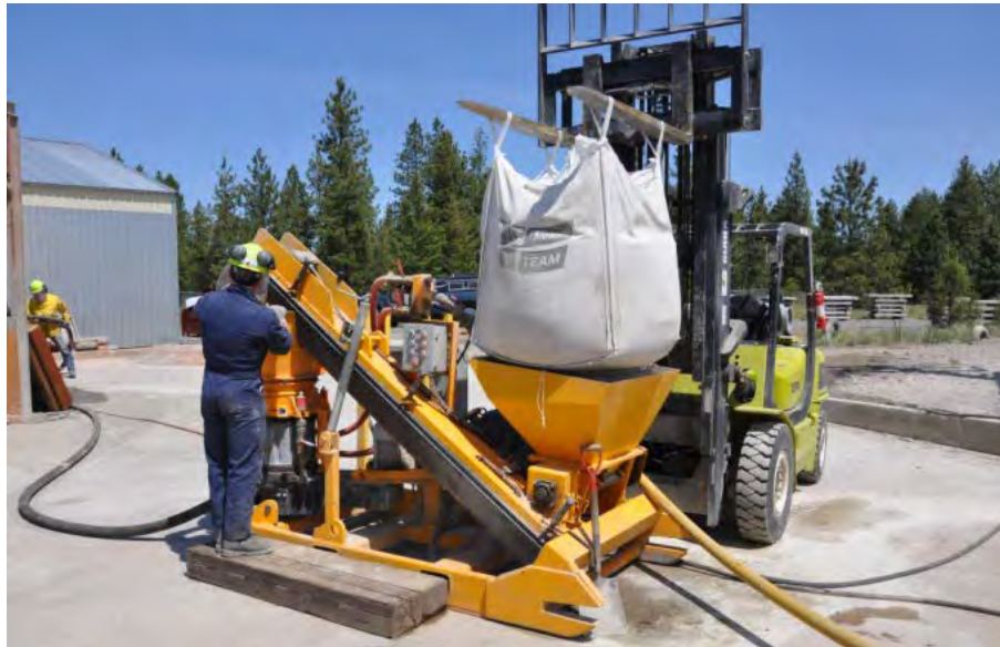
Figure 28. Operation of a dry mix shotcrete machine equipped with a rotary barrel.
