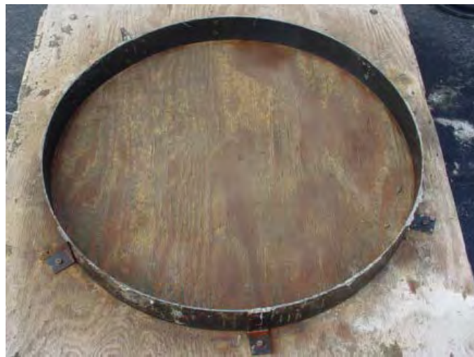
Figure 75. Mold ring used to prepare a round-panel shotcrete sample.
