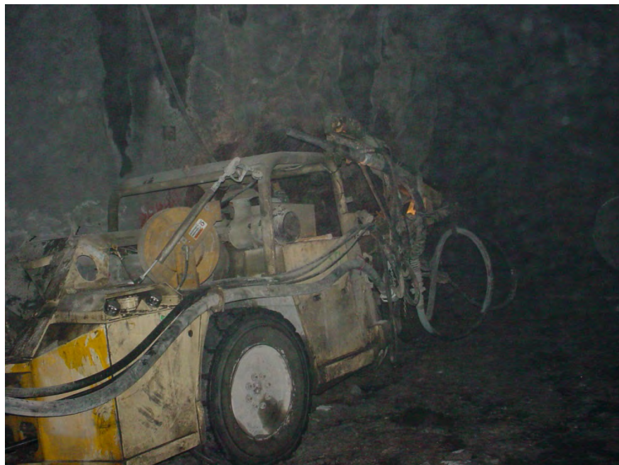
Figure 30. Operation of a wet mix shotcrete machine.
