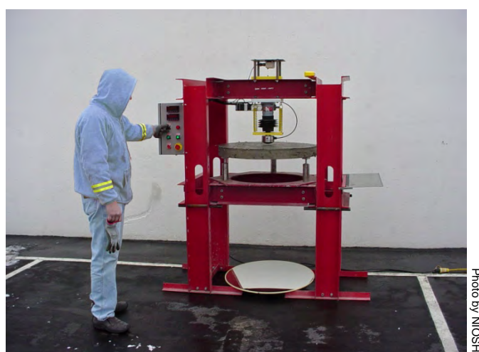
Figure 74. Operation of portable round determinate panel (RDP) test machine.
