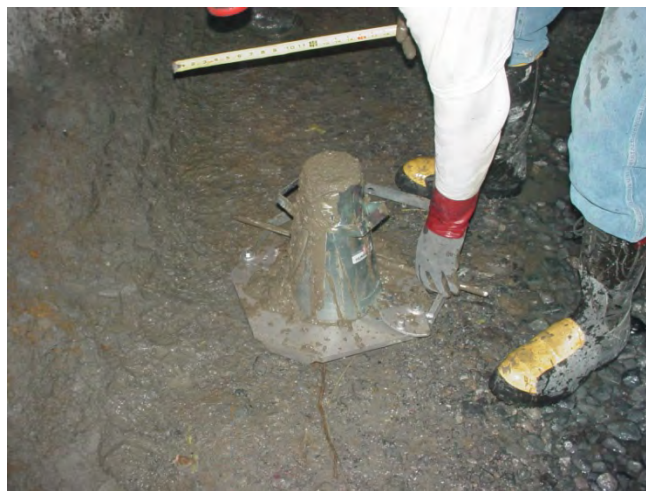
Figure 32. Filling a slump cone with wet mix shotcrete prior to conducting a slump test in an underground mine.
