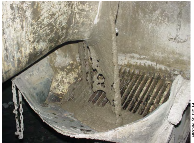
Figure 31. Consistency of wet mix shotcrete being loaded into the hopper of a shotcrete machine.
