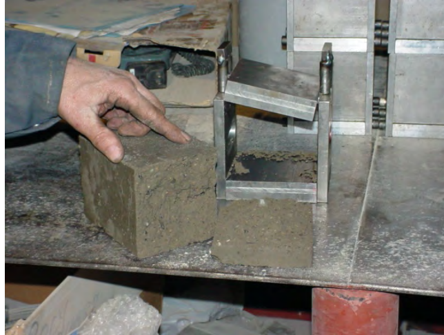
Figure 50. Shotcrete sample showing exposed failure plane.
