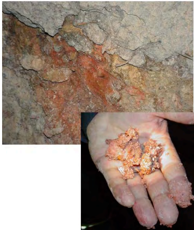
Figure 3. Poor-quality, highly deformable rock in an underground gold mine in Nevada.
