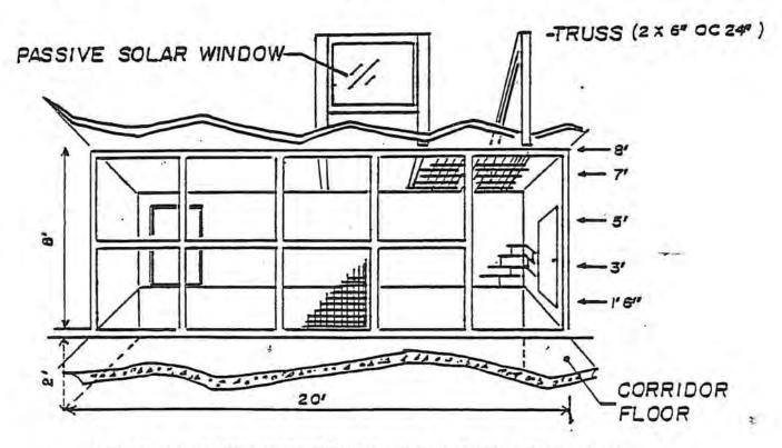
CUT-AWAY VIEW OF REPRESENTATIVE CAGE SHOWING HEIGHT ABOVE CORRIDOR FLOOR WHERE CH2O WAS MEASURED
