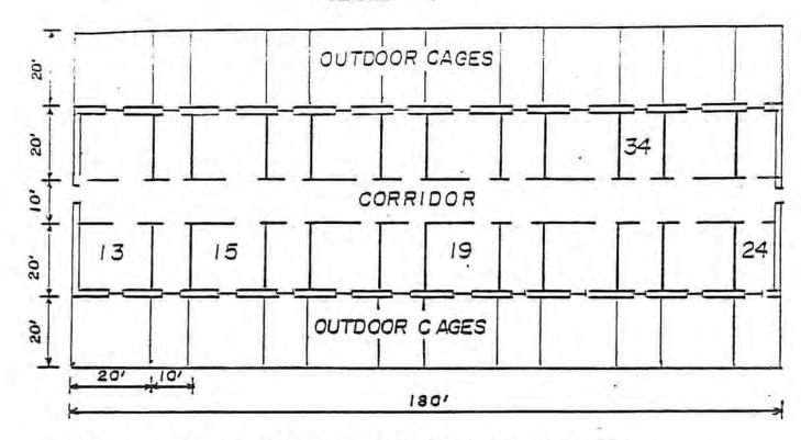
FLOOR PLAN OF SMALL ANIMAL FACILITY. NUMBERS INDICATE CAGES WHERE CH2O WAS MEASURED.
