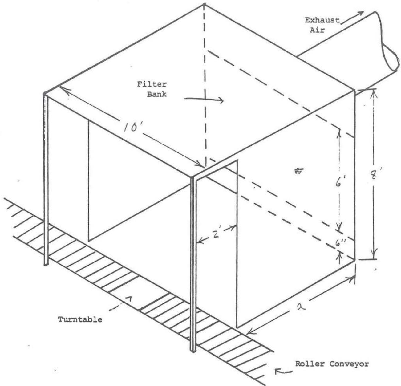
FIGURE 2: General Layout of the Spray Finishing Booths
