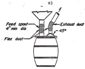
Q=50 cfm × drum dia (ft) for weighted lid 150 cfm × drum dia (ft) for loose lid Duct velocity = 3500 fpm minimum Entry loss = 0.25 VP
