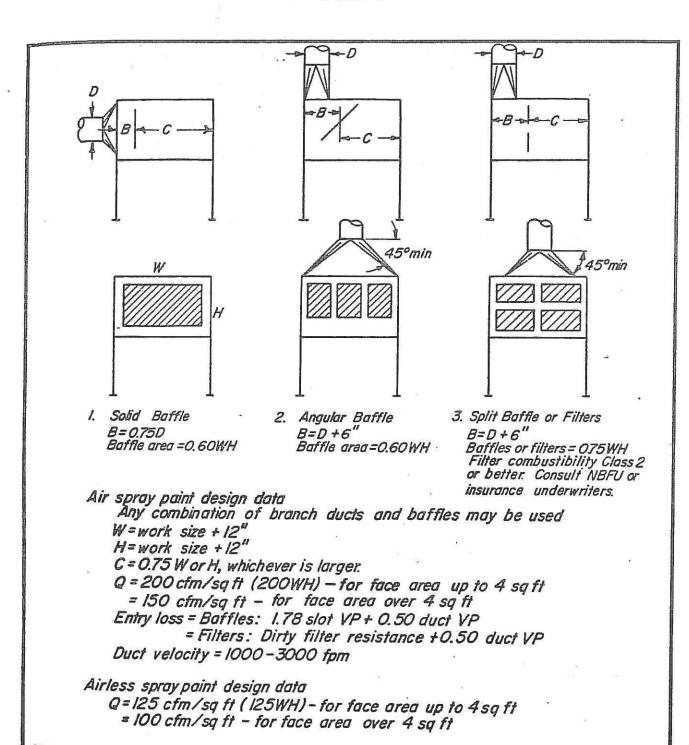
Note: Baffle arrangements shown are for air distribution only. Filters and/or other air cleaning devices may be required to meet air pollution codes or local conditions.
