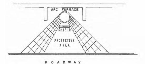
Figure 2: Schematic diagram of locations (shaded area) where optical radiation levels were measured.
