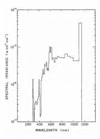
Figure 5: Maximum, minimum, and average variation in spectral irradiance at selected UV wavelengths.
