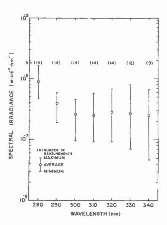
Figure 4: Spectral irradiance values (cosine corrected) of 1700 kW electric arc furnace 5 hours after start-up. Measured total spectral irradiance from 280-1100 nm is 5.5 mW·cm<sup>-2</sup> at 4.6 m. Note bandwidth changes. Furnace temperature approximately 1900°C.
