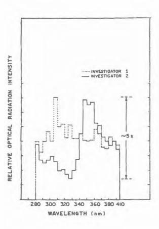
Figure 3: Variation in optical radiation levels. Two scans performed by different investigators on same arc event. The scans, requiring two minutes each to complete, were separated by a time interval of one minute.
