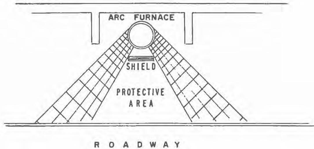
Figure 2: Schematic diagram of locations (shaded area) where optical radiation levels were measured.
