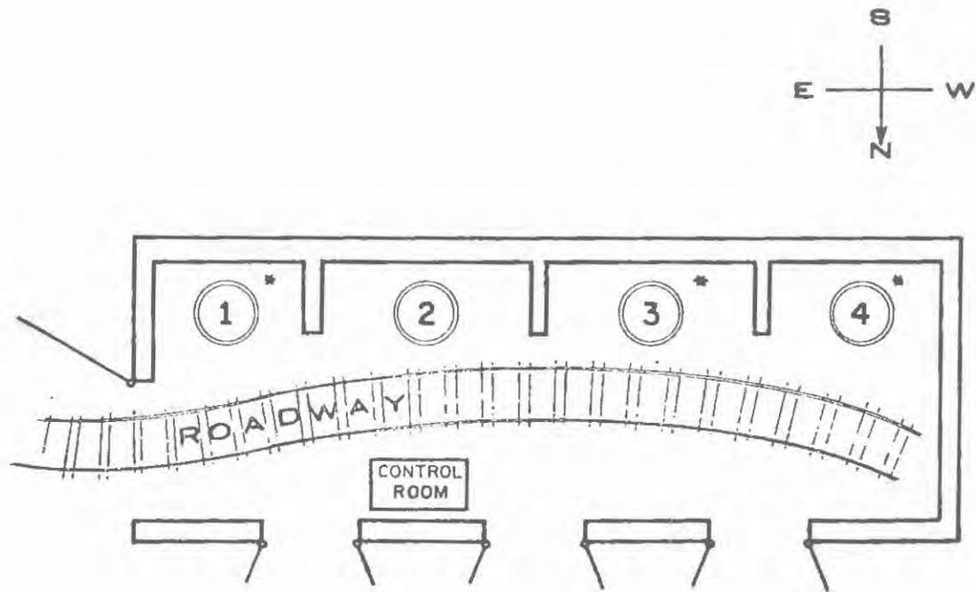
Figure 1: Layout of arc furnaces. The asterisks indicate operating furnaces during the study.
