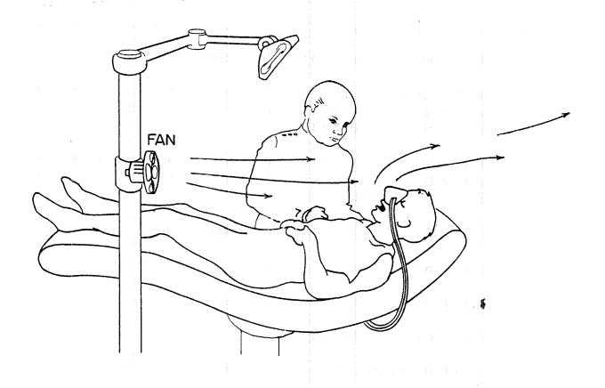
NOTE: The apparatus consist of a quietly operating fan located to take in relatively fresh air.
