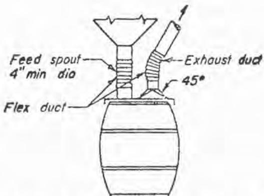
$Q = 50 \text{ cfm} \times \text{drum dia (ft)}$  for weighted lid
