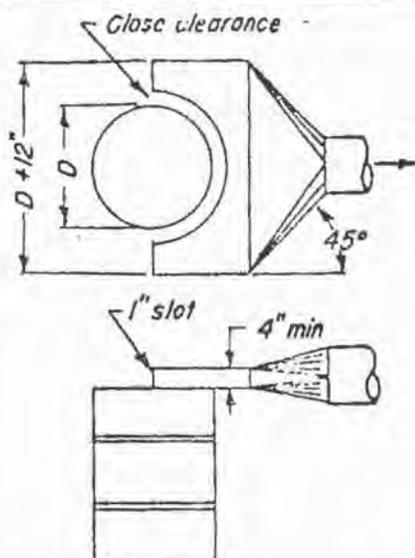
$Q = 100 \text{ cfm/sq ft barrel top min}$
