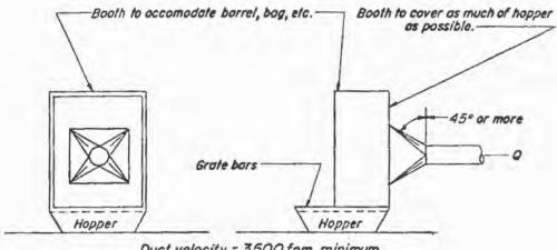
Duct velocity = 3500 fpm minimum Q = 150 cfm/sq ft face Entry loss = 0.25 VP
