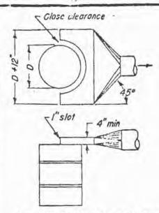
Q = 100 cfm/sq ft barrel top min Duct velocity = 3500 minimum Entry loss = 0.25 VP + 1.78 slot VP Monual loading.
