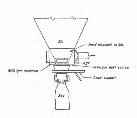
Q = 400 - 500 cfm - non-toxic dust 1000 - 1500 cfm - toxic dust Duct velocity = 3500 fpm minimum Entry loss = 0.25 VP
