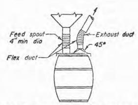
Q = 50 cfm × drum dia (ft) for weighted lid 150 cfm × drum dia (ft) for loose lid Duct velocity = 3500 fpm minimum Entry loss = 0.25 VP
